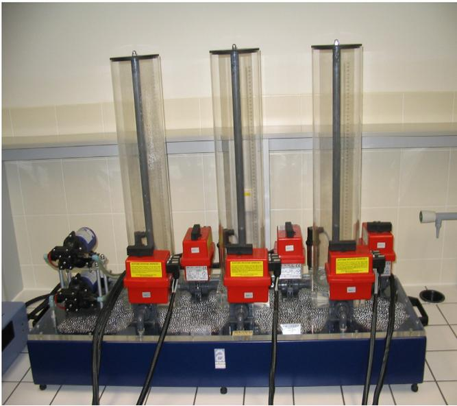
Fig. 1. Amira DTS200 – three tank system
