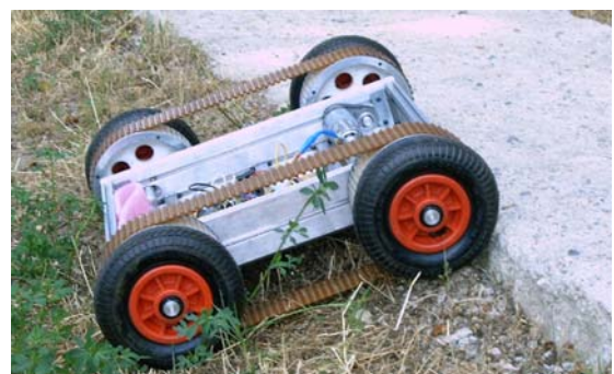
Fig. 7 Manufactured reconfigurable mobile platform
