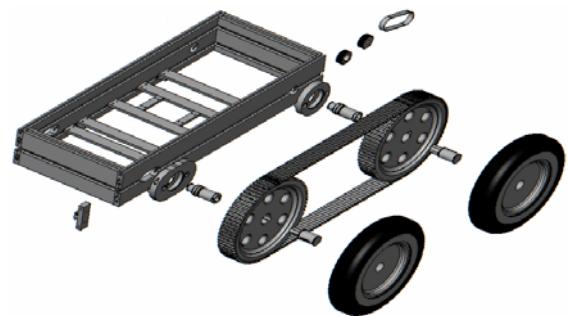
Fig. 6 Exploded view of the robot's configurable driving systems
