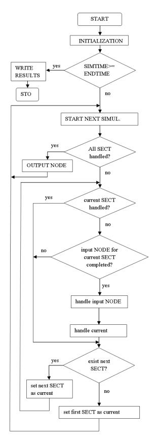
Fig. 9 Block diagram for class SIMULATOR
