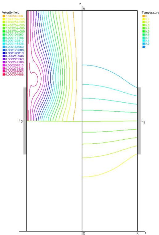
Fig. 11. Streamlines and temperature profile for  $L_g = 0.375$ ,  $Ra = 10^3$ .
