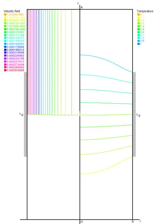
Fig. 5. Streamlines and temperature profile for  $L_g = 0.500$ ,  $Ra = 0$ .
