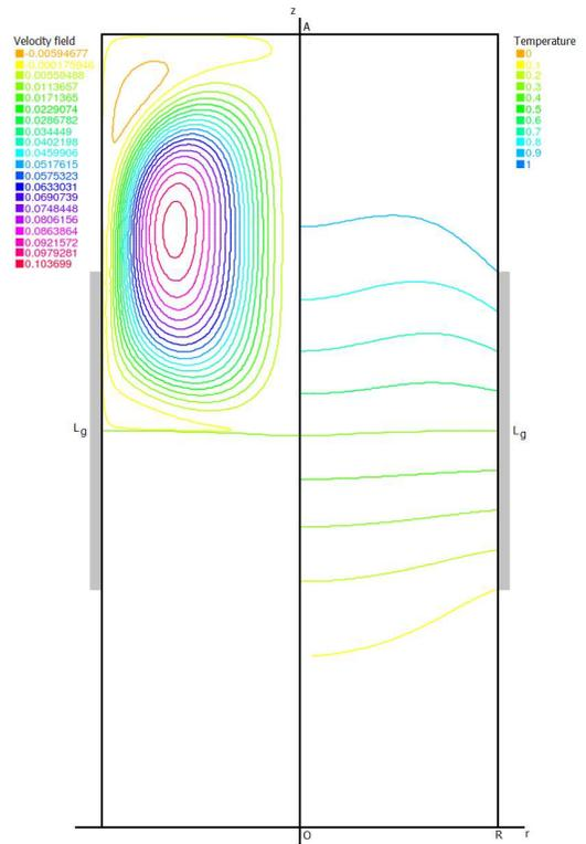
Fig. 19. Streamlines and temperature profile for  $L_g = 0.500$ ,  $Ra = 10^6$ .
