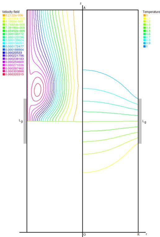
Fig. 10. Streamlines and temperature profile for  $L_g = 0.250$ ,  $Ra = 10^3$ .
