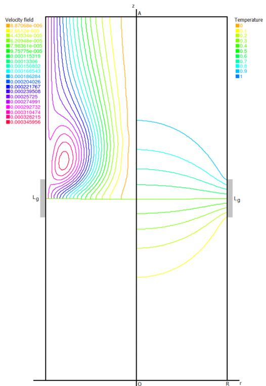
Fig. 9. Streamlines and temperature profile for  $L_g = 0.125$ ,  $Ra = 10^3$ .
