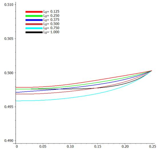
Fig. 8. The solidification interface corresponding to different values of  $L_g$ , for  $Ra = 0$
