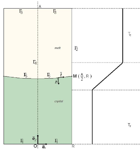
Fig. 1. The computational domains and the temperature profile inside the furnace
