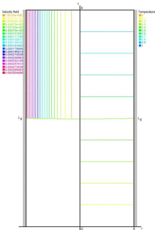
Fig. 14. Streamlines and temperature profile for  $L_g = 1.000$ ,  $Ra = 10^3$ .
