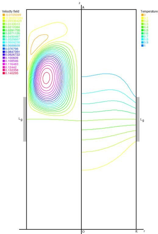
Fig. 17. Streamlines and temperature profile for  $L_g = 0.250$ ,  $Ra = 10^6$ .
