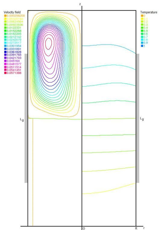
Fig. 20. Streamlines and temperature profile for  $L_g = 0.750$ ,  $Ra = 10^6$ .
