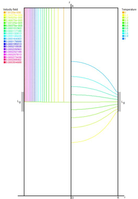
Fig. 2. Streamlines and temperature profile for  $L_g = 0.125$ ,  $Ra = 0$ .
