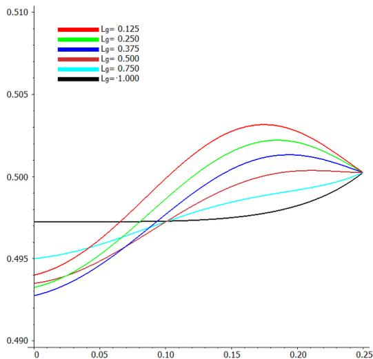
Fig. 22. The solidification interface corresponding to different values of  $L_g$
