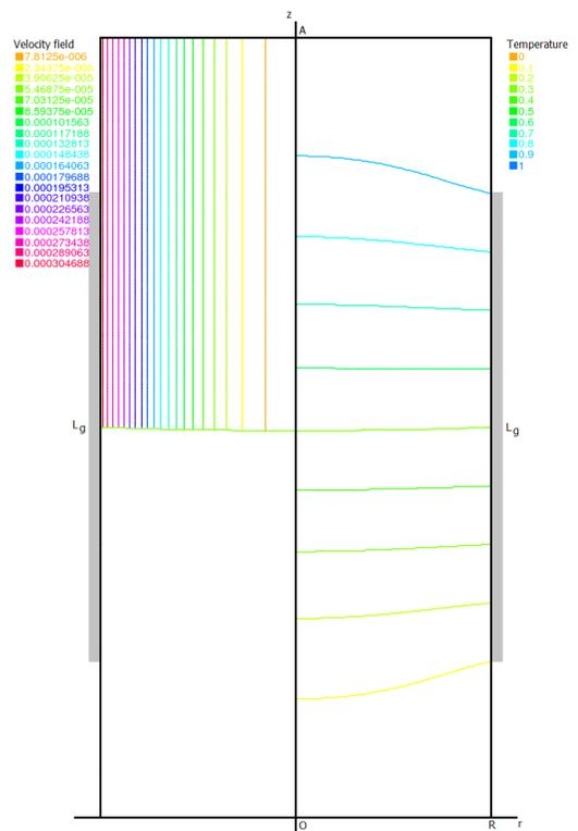
Fig. 6. Streamlines and temperature profile for  $L_g = 0.750$ ,  $Ra = 0$ .
