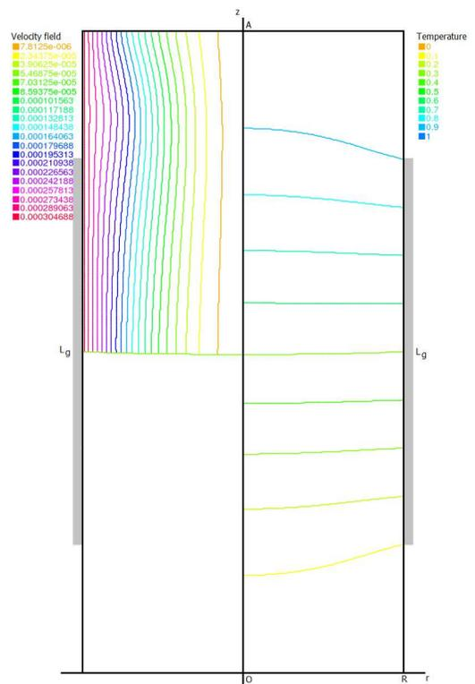
Fig. 13. Streamlines and temperature profile for  $L_g = 0.750$ ,  $Ra = 10^3$ .
