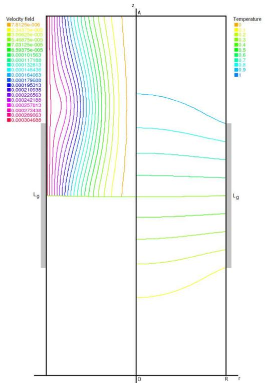
Fig. 12. Streamlines and temperature profile for  $L_g = 0.500$ ,  $Ra = 10^3$ .
