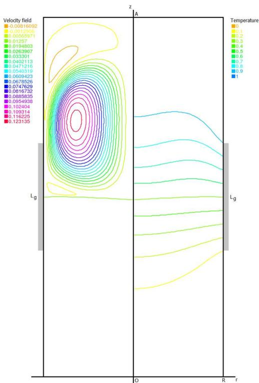
Fig. 18. Streamlines and temperature profile for  $L_g = 0.375$ ,  $Ra = 10^6$ .
