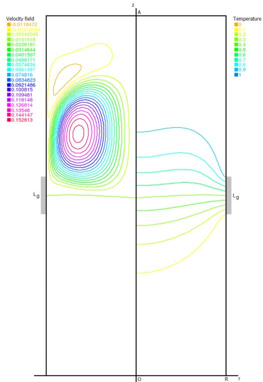
Fig. 16. Streamlines and temperature profile for  $L_g = 0.125$ ,  $Ra = 10^6$ .
