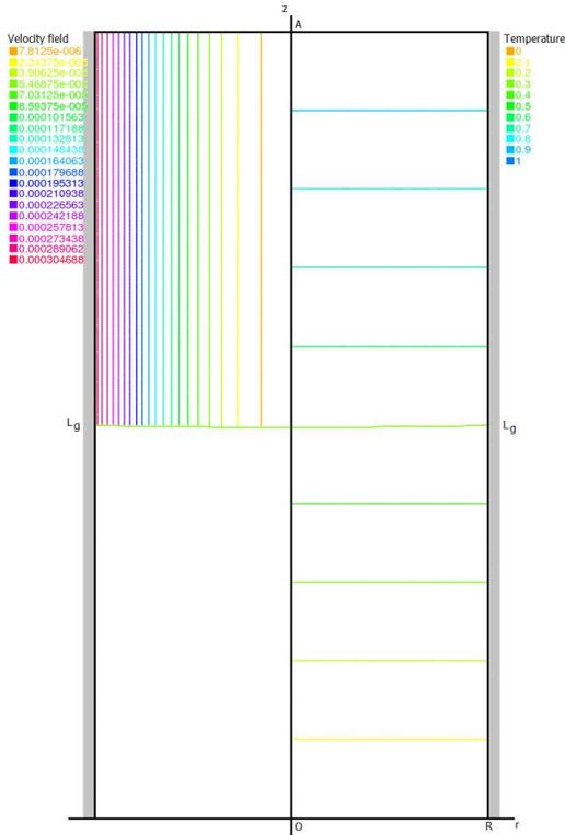
Fig. 7. Streamlines and temperature profile for  $L_g = 1.000$ ,  $Ra = 0$ .
