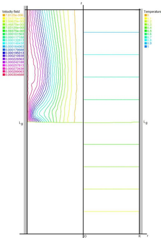
Fig. 21. Streamlines and temperature profile for  $L_g = 1.000$ ,  $Ra = 10^6$ .
