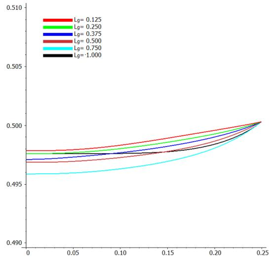
Fig. 15. The solidification interface corresponding to different values of  $L_g$  for  $Ra = 10^3$
