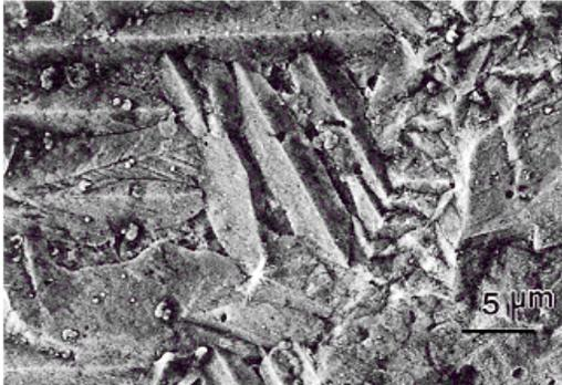
Fig. 2. Details of surface needle growth of  $\gamma'$ -Fe<sub>4</sub>N<sub>1-x</sub> by branching
