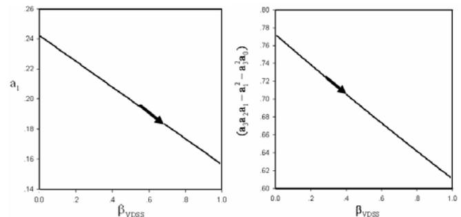
Fig. 4 The second and fourth conditions which satisfies the Routh-Hurwitz criteria. The value of parameters are defined in Table 2.
