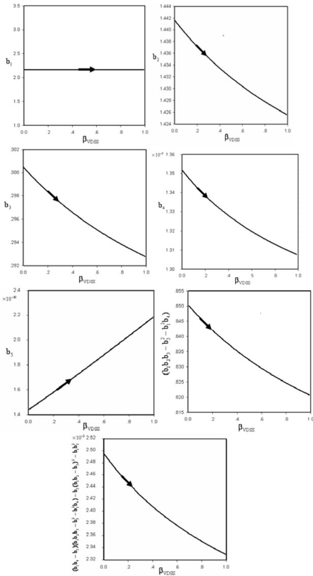
Fig. 5 The three above conditions which satisfies the Routh-Hurwitz criteria. The value of parameters are defined in Table 2.
