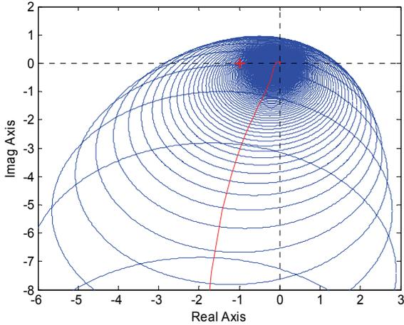
Fig. 9 graphical interpretation of stability condition (14) for controller (21) – robustly unstable case
