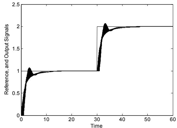
Fig. 13 output signals of 91 “representative” systems for the controller (22) – robustly stable case
