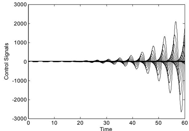
Fig. 12 control signals going from the controller (21) to 91 “representative” systems – robustly unstable case
