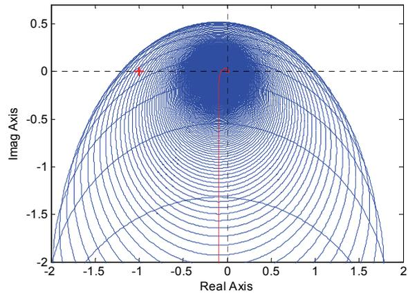
Fig. 15 graphical interpretation of stability condition (14) for controller (29) – robustly ?unstable? case
