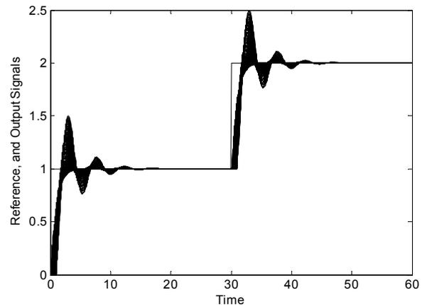
Fig. 16 output signals of 91 “representative” systems for the controller (29) – robustly ?unstable? case
