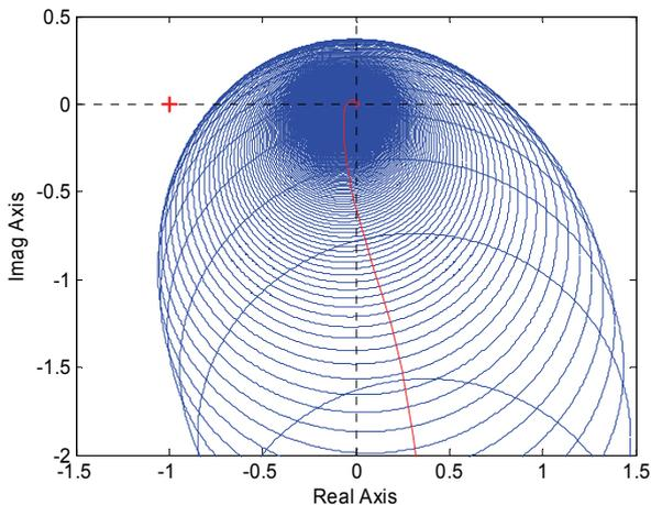
Fig. 10 graphical interpretation of stability condition (14) for controller (22) – robustly stable case
