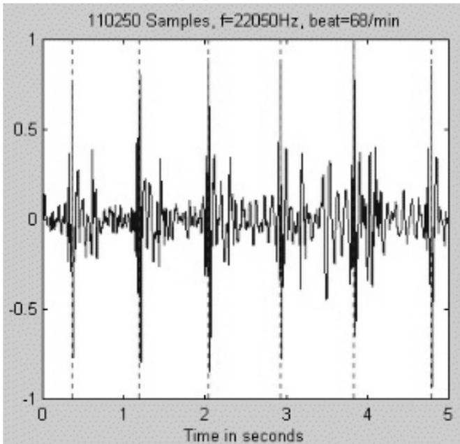
Fig. 8 Signal at the output of the microphone [6]
