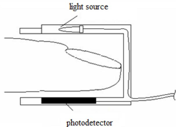
Fig. 4 Translucent method of heart rate scanning [3]
