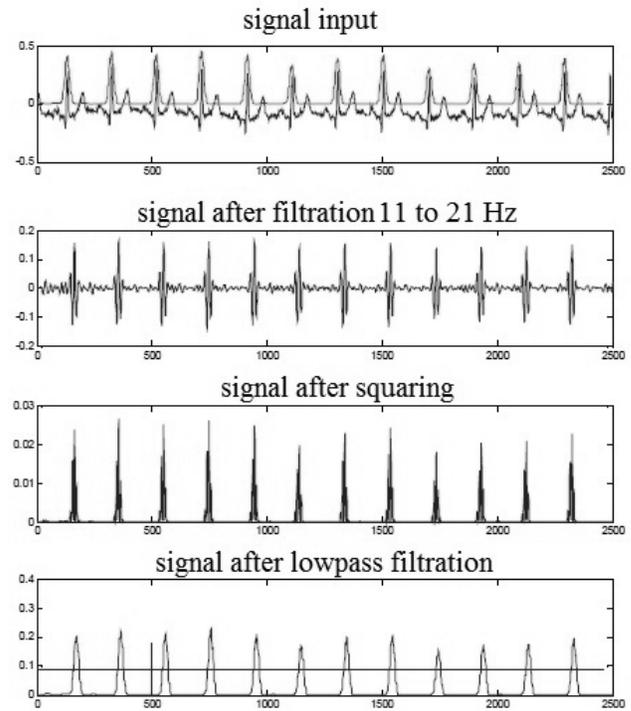
Fig. 12 Detection of the QRS complex [1]
