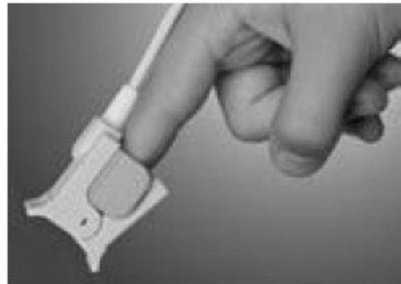
Fig. 3 Optical sensor of heart rate [16]
