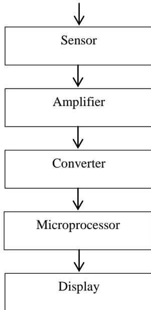
Fig. 2 General block diagram of the heart rate measurement
