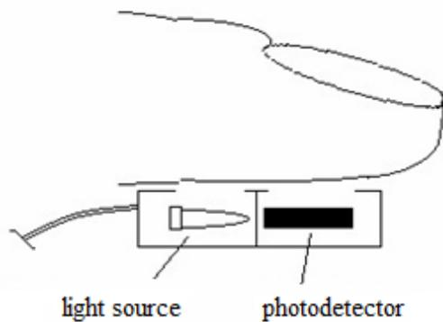
Fig. 5 Reflexion method of scanning [3]
