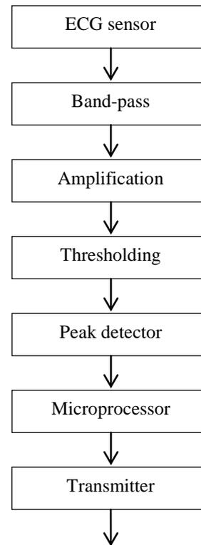
Fig. 11 Block diagram of the R wave detector
