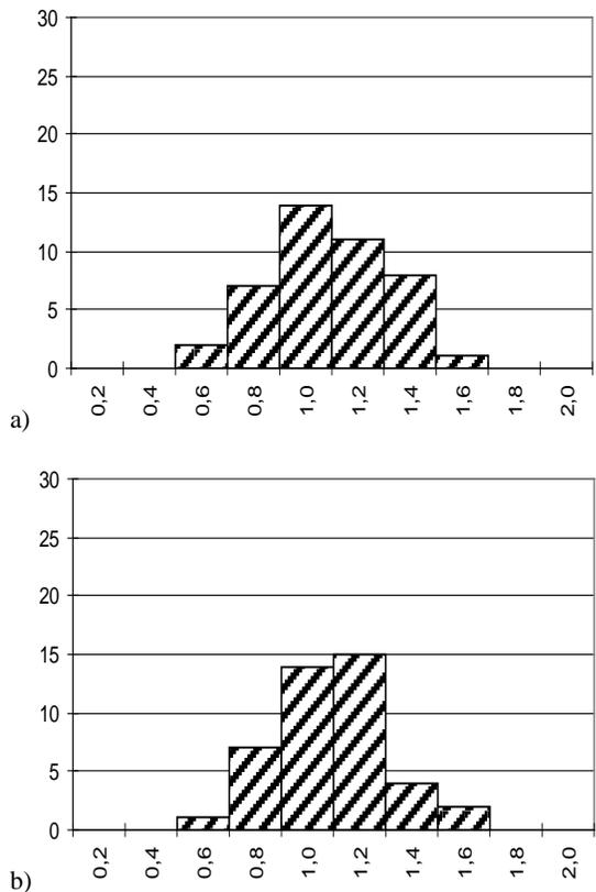
Fig. 8 shear loading – histogram of  $V_{u,ex} / V_{um}$  ratios:
