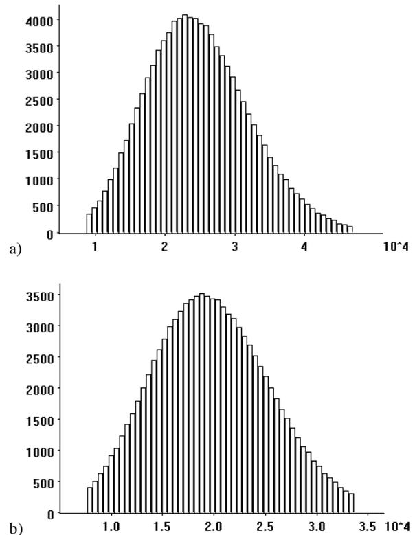
Fig. 10 Shear loading – examples of MC-simulation of  $V_{ud}$ : a)  $V_{ud}$  according to (22), b)  $V_{ud}$  according to (24)
