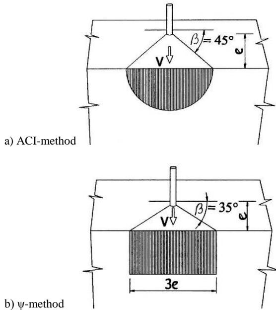
Fig. 5 shear loading – lateral concrete-cone failure: principles of calculating methods
