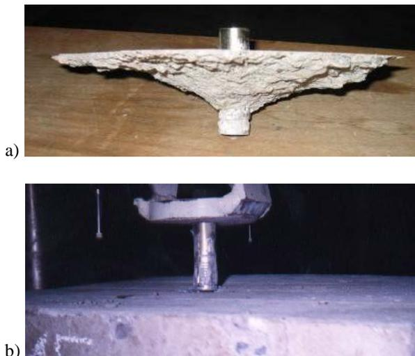
Fig. 2 tensile loading – illustration of actual concrete failure modes: a) concrete-cone failure, b) anchor pull-out
