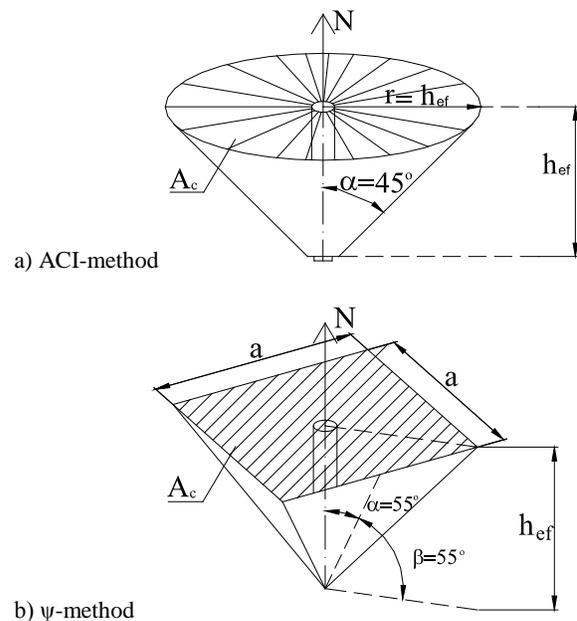
Fig. 3 tensile loading – concrete-cone failure: principles of calculating methods
