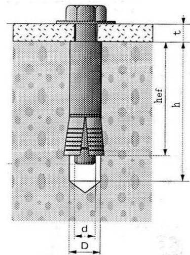
Fig. 1 typical composition of torque-controlled expansion anchor
