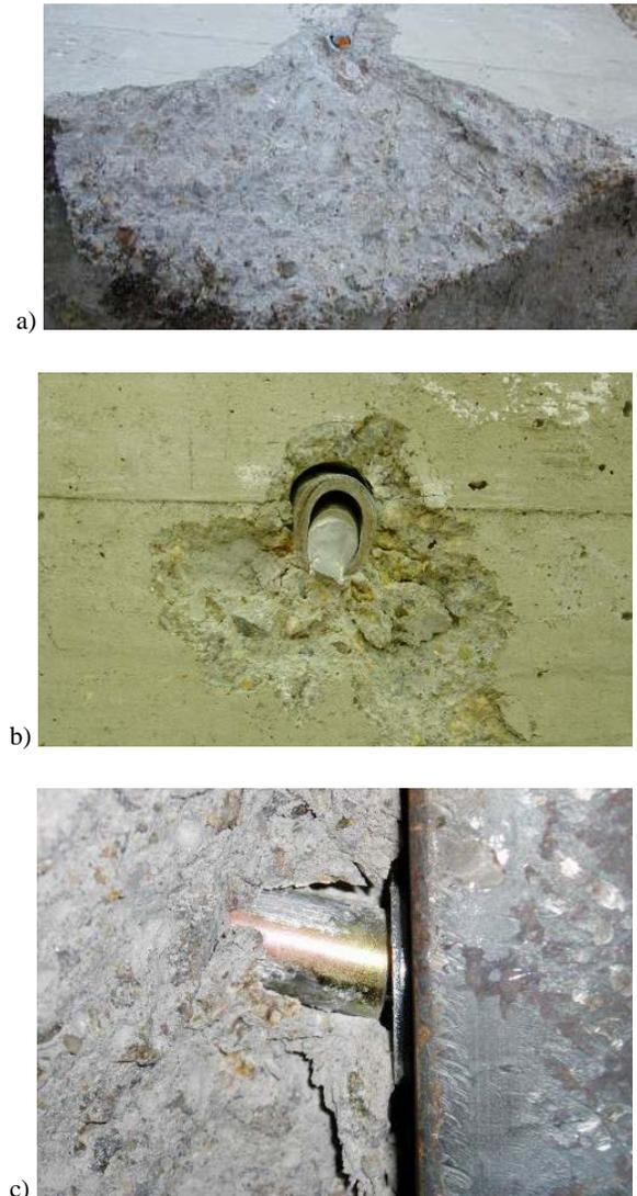
Fig. 4 shear loading – illustration of actual concrete failure modes:
