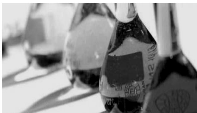
Fig. 3 Increasing (from left to right) color intensity of resulting solutions caused by increasing an amount of CrVI in these solutions
