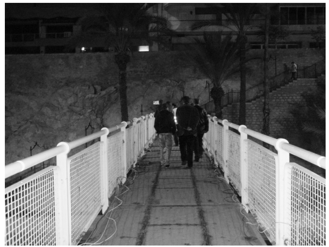
Fig. 8 Test on the footbridge. Disposition of the pedestrian stream.
