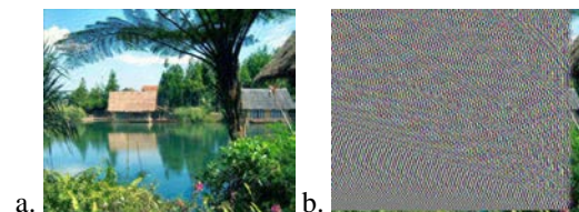
Fig. 5 a. Result of inverse filtering opposed to b. The naive method in deblurring with a complicated PSF
