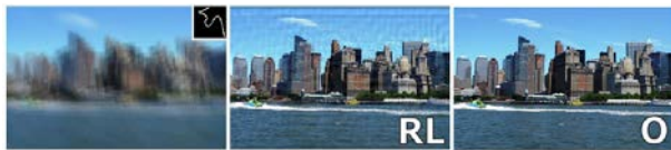
Fig. 11 From left to right: input blurred image; recovered image with Richardson-Lucy algorithm; the RL result cleaned with the mentioned algorithm. Image from “ Dual range deringing for Non-blind image deconvolution ” [9]
