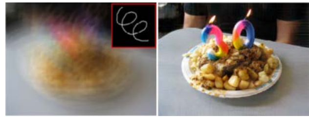
Fig. 12 Left: input blurred image and kernel; right: result of interscale-intrascale algorithm. Image from “ Progressive Inter-Scale Non-Blind Image Deconvolution ” [8]
