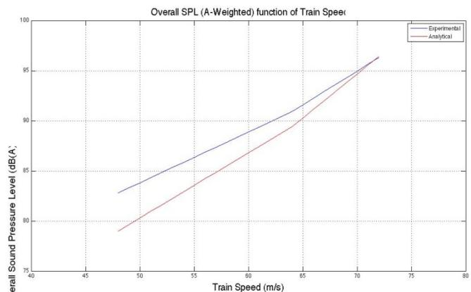
Fig. 18: Experimental and Analytical Overall SPL(dB(A)) function of train speed
