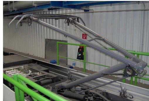
Fig. 5 – Typical "half-pantograph" configuration
