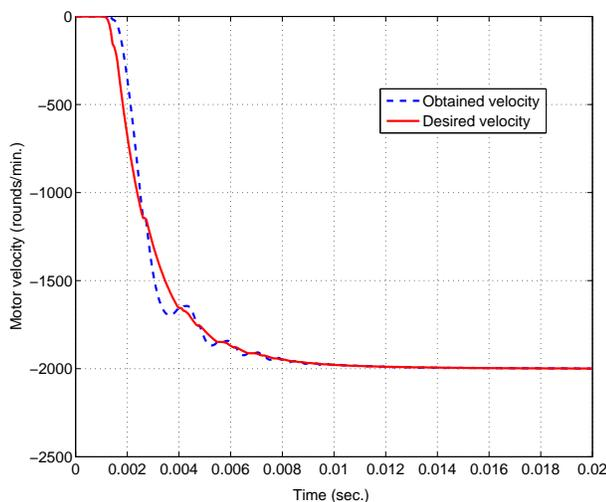
Fig. 6. Profile of the obtained and desired motor velocity using a maximal switching chopper frequency equals 2.5 kHz in case of negative desired velocity
