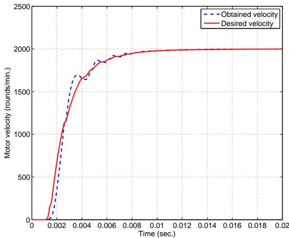
Fig. 5. Profile of the obtained and desired motor velocity using a maximal switching chopper frequency equals 2.5 kHz in case of positive desired velocity
