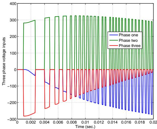
Fig. 9. Three-phase control signals after the chopper controller using a PWM signal with a maximal switching frequency equals 2.5 kHz in case of positive desired velocity
