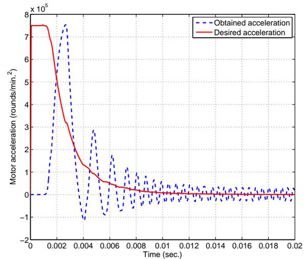
Fig. 7. Profile of the obtained and desired motor acceleration using a maximal switching chopper frequency equals 2.5 kHz in case of positive desired velocity
