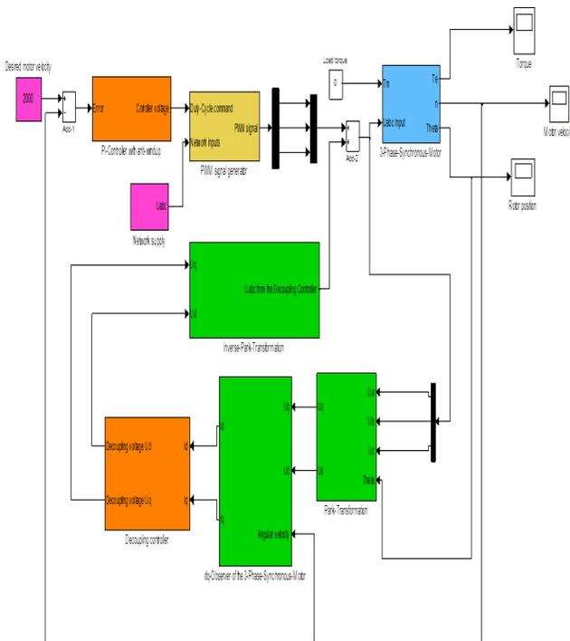
Fig. 2. Simulink structure of the whole control system
