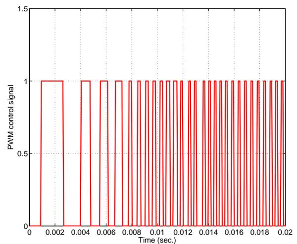
Fig. 8. PWM signal used as a chopper with a maximal switching frequency equals 2.5 kHz in case of positive desired velocity
