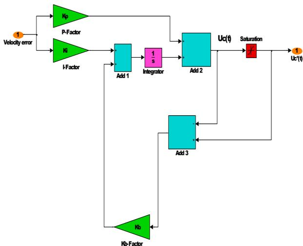
Fig. 3. Simulink structure of PI controller including anti-windup scheme
