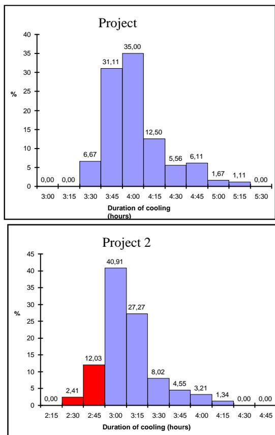
Fig. 1. Durations of casting cooling in a mould distribution.
