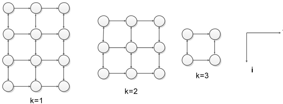
Fig. 8. Dependence graph of the systolic array for QR decomposition using householder reflections
