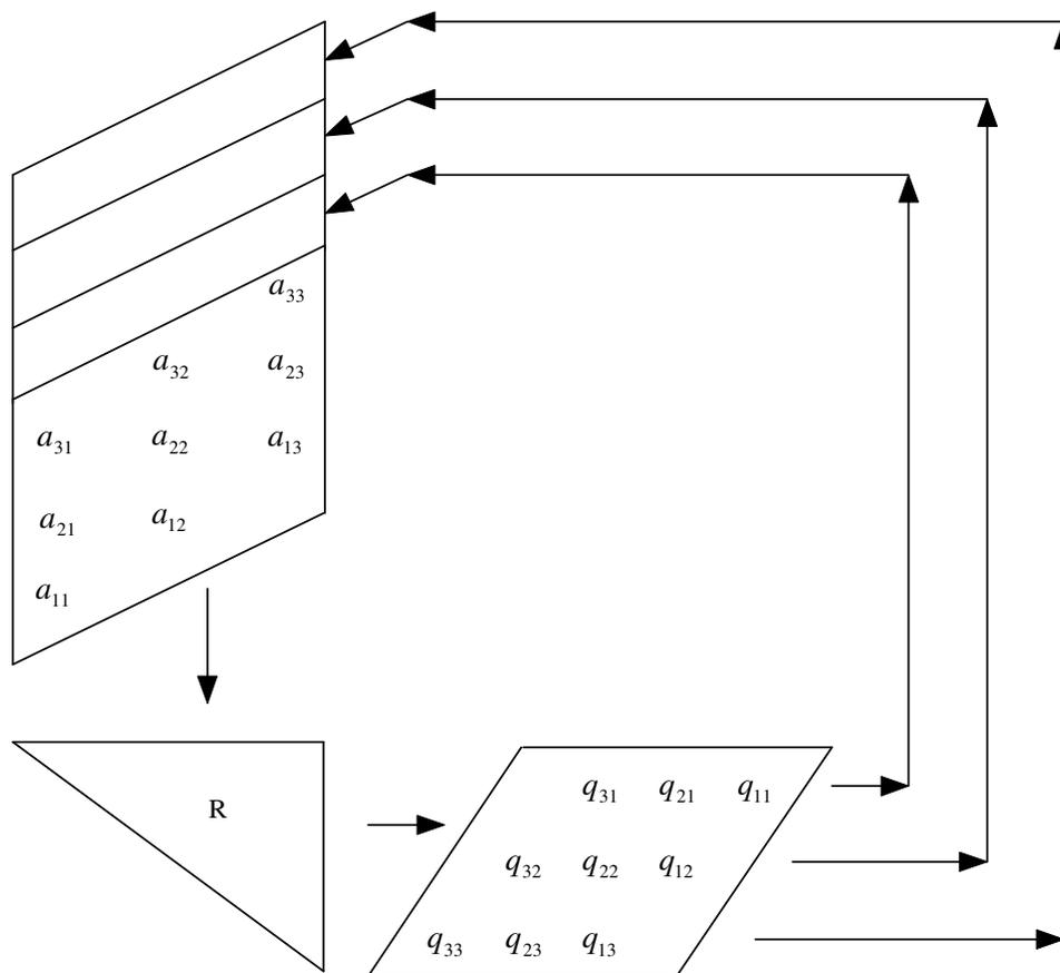
Fig. 5 Systolic model for computing the Q matrix
