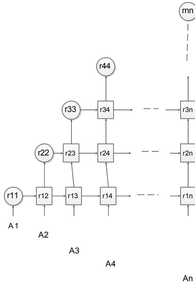
Fig. 9. Systolic array for parallel QR decomposition using householder reflection
