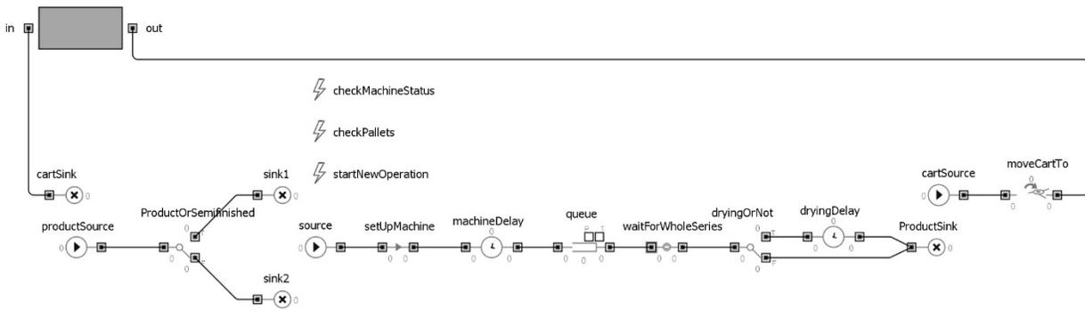
Figure 3: Schematic of a single machine in the DES model
