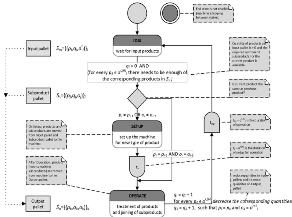
Figure 2: UML state diagram of a single machine
