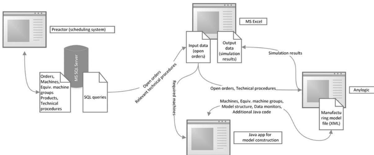
Figure 4: Simulation system schematics
