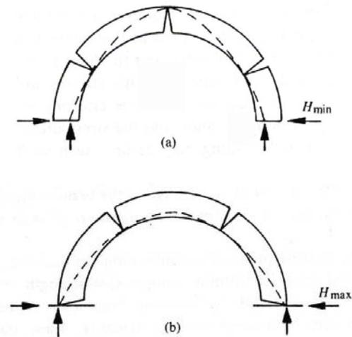
Fig.1 (a) Minimum abutment thrust (b) Maximum abutment thrust
