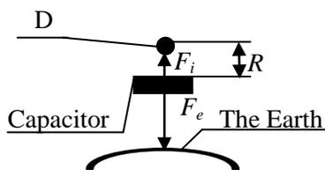
Fig.2. The forces of interaction of the body D,  $i$ -th capacitor and the Earth.
