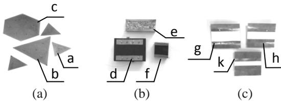
Fig 1. Deployed capacitors on fiberglass (a), granite (b) and ceramic (c) substrate used during the experiments (top view)
