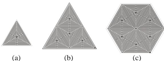
Fig. 3. Geometry of electrodes in the first group of capacitors
