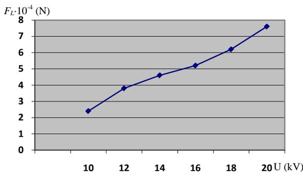
Fig. 9. Lifting force  $F_L$  on voltage  $U$  dependence if  $\alpha = \alpha_{opt}$ .
