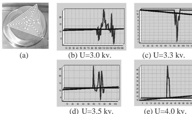
Fig. 5. Alumina based ceramic sample on the weight table (a), and its’ weight change under different voltage (b – e).
