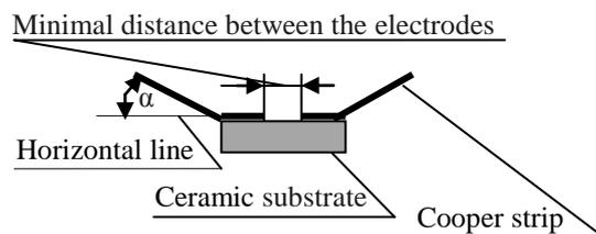
Fig 7. Construction of deployed capacitors on ceramic substrate used during the third series of experiments (butt view).
