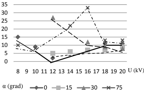
Fig. 8. Distances  $R_h$  values as functions on voltage  $U$  and on angle  $\alpha$ .
