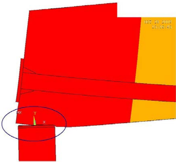
Fig. 10 Placing the beam on a reinforced concrete structure – deformation u_v [mm]
