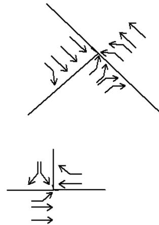
Fig. 12 Signalized access with allowed left turns and 2-out lanes and new additional access
