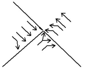
Fig. 9 Signalized access with allowed left turns and 2-out lanes
