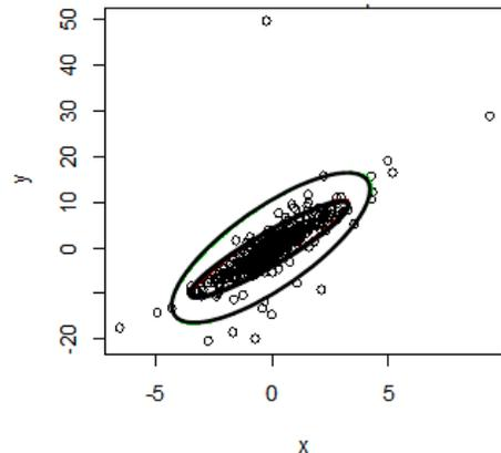
Fig. 17 Minimum covariance determinant estimator. Access design 5
