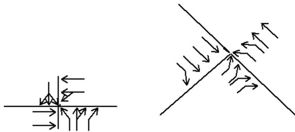
Fig. 11 Two signalized accesses with allowed left turns and 4-out lanes
