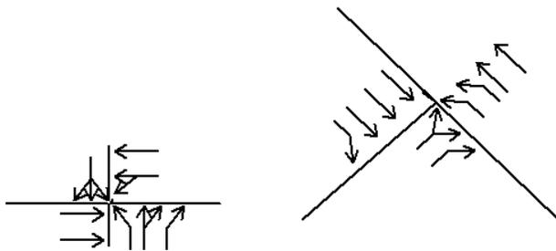
Fig. 10 Two Signalized accesses with allowed left turns and 2-out lanes in T-lane intersection
