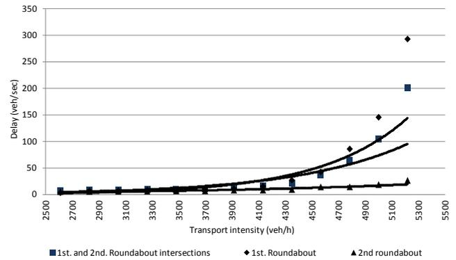
Fig. 5 Delay at intersection system with two roundabout intersections
