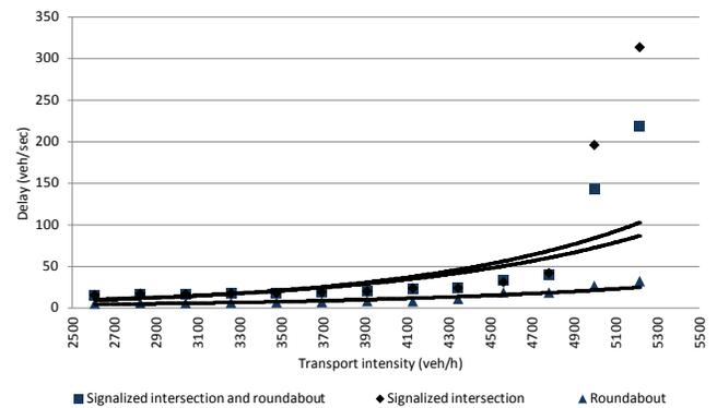
Fig. 6 Delay at intersection system with two intersections (signalized with left shoulder and roundabout)
