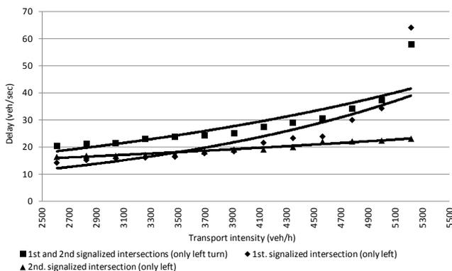
Fig. 4 Delay at intersection system with two signalized intersections (left turn from shoulder)
