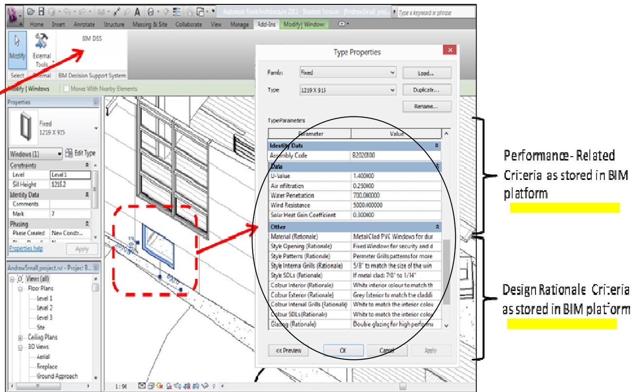
Fig. 4: BIM setup with design rationale
