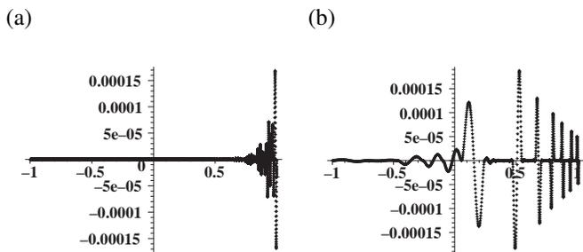
Fig. 5. Plots of the errors approximation of the function  $\sin(\exp(3x))$ , when (a)  $x_{j+1} = x_j + h$ ,  $h = 1/50$ ,  $n = 100$ , and (b) when  $h_0 = 0.28$ ,  $h_j$  we obtain from (11),  $n = 48$
