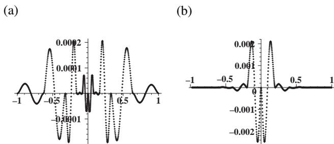
Fig. 6. Plots of the errors of approximation of the Runge function, when (a)  $n = 10$ ,  $h_i$  we obtain using (11),  $j = 0, 1, 2, 7, 8, 9$ ,  $x_{j+1} = x_j + h_j$ ,  $h_j = h_2/2$ ,  $j = 3, 4, 5, 6$ , and (b)  $n = 10$ ,  $x_{j+1} = x_j + h_j$ ,  $h_j = 0.2$ ,
