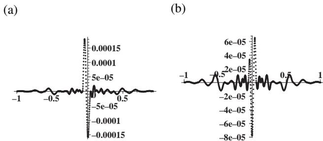
Fig. 4. Plots of the errors of approximation of the Runge function,  $h_j$  we obtain from (11),  $n = 15$ , when (a)  $h_0 = 0.2$ , (b)  $h_0 = 0.205$
