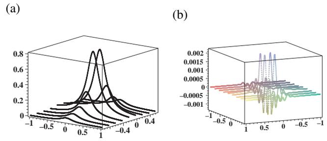
Fig. 20. Plots of the approximation of the function  $u_3 = 1/((1+25x^2)(1+25y^2))$  (a), and the error of approximation of the function  $u_3$  (b), here  $h = 0.2$ ,  $\Omega = [-1, 1] \times [-1, 1]$
