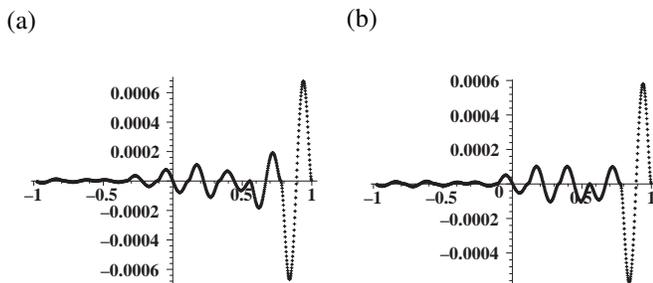
Fig. 11. Plots of the errors of approximation of the function  $15 \cos(2x) \sin(\exp(x))$  with the polynomial splines (a), and with the trigonometrical splines (b)
