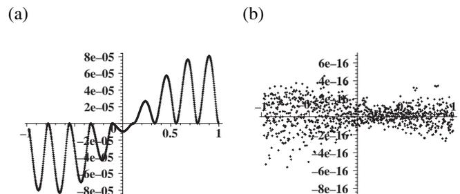
Fig. 16. Plots of the errors of approximation of the function  $7 \cos(2x) + 5 \sin(x)$ : (a) with the polynomial splines, and (b) with the trigonometrical splines
