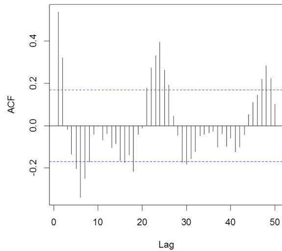
**Fig. 29:** Correlogram of the wind speed series after performing the first order difference. The value of autocorrelation coefficient is plotted as a function of the lag.
