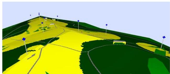
**Fig. 20:** 3D noise map of the wind farm area obtained in CadnaA®. The Source Power level is 97.4 dBA.
