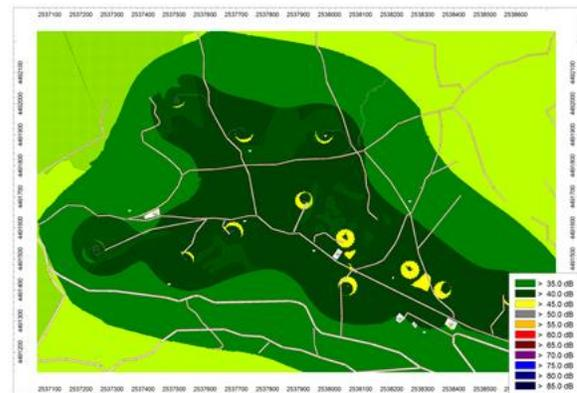
**Fig. 19:** Noise map of the wind farm area. Source Power Level: 93.4 dBA.
