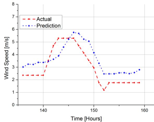
**Fig. 31:** Wind speed in the 24 validation hours. The red dashed line shows the actual data, the green dotted line shows the prediction. All the data are hourly mean in meters per second.
