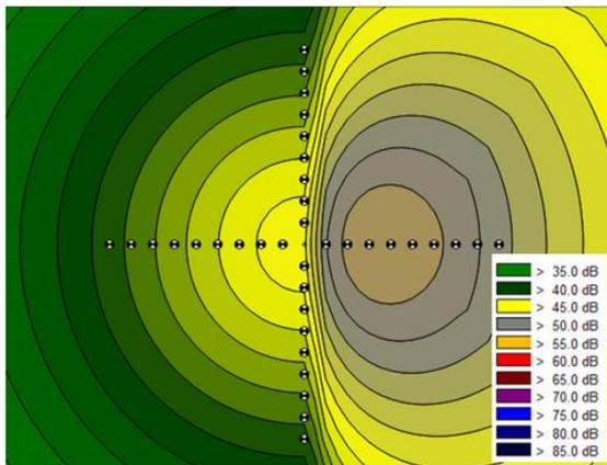
**Fig. 4:** CadnaA® noise map (values are in dBA) for a pointlike source with  $L_w=98$  dBA, height=70 m with high directivity.
