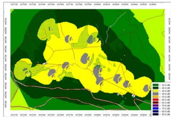
**Fig. 25:** Noise map of the wind farm area. Source Power Level: 98.3dBA, with a preferred direction: WNW.
