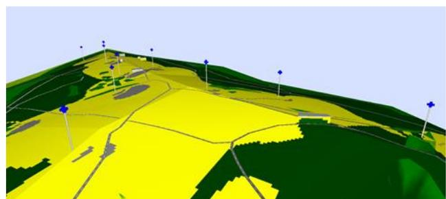
**Fig. 27:** 3D noise map of the wind farm area obtained in CadnaA®. The source power is 97.4 dBA with directivity.
