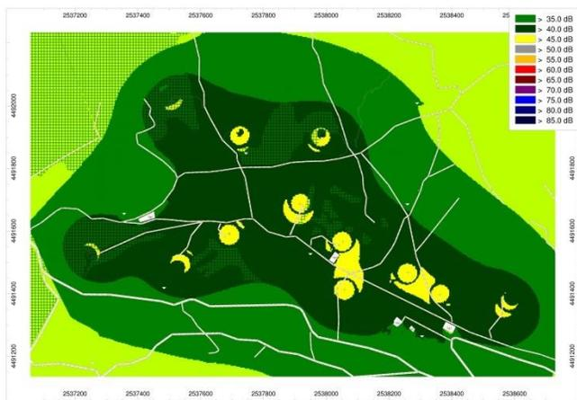
**Fig. 32:** Noise map of the wind farm area, with average wind speed predicted by the SARIMA model. Source Power Level: 94.6 dBA.
