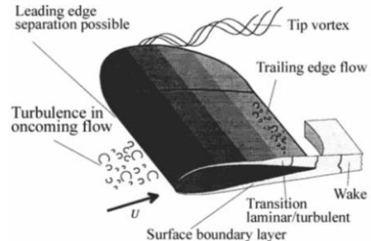
Fig. 2: Schematic of flow around rotor blade [8].
