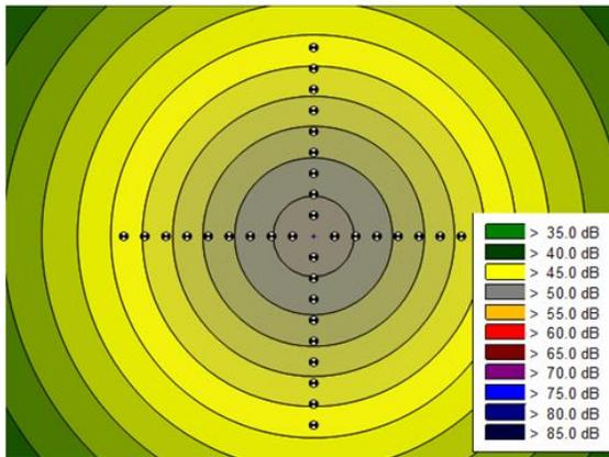
**Fig. 3:** CadnaA® noise map (values are in dBA) for a pointlike source with  $L_w=98$  dBA, height=70 m.
