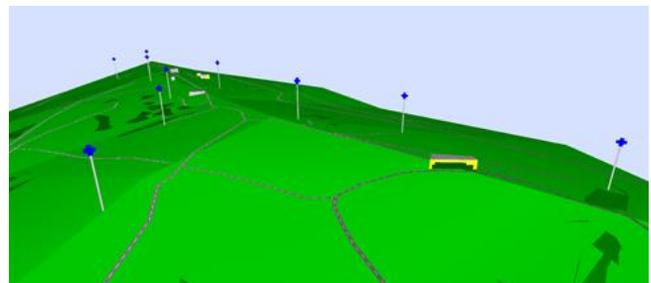
**Fig. 7:** 3D view of the wind farm area of Taverne Vecchie, implemented on CadnaA®. The blue crosses are the pointlike sources simulating the wind turbines.
