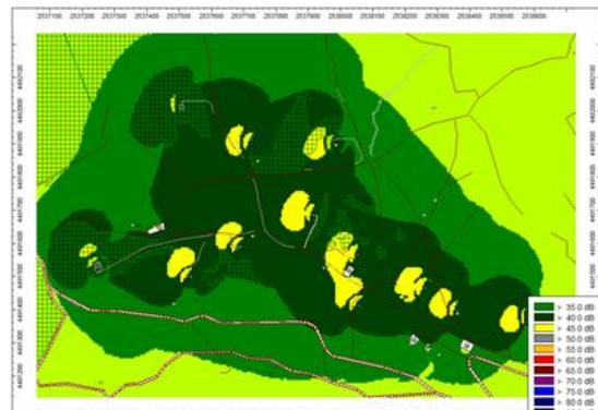
**Fig. 26:** Noise map of the wind farm area. Source Power Level: 93.4 dBA, with a preferred direction: WNW.
