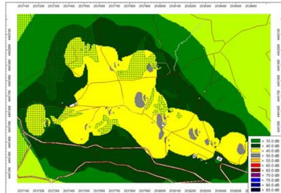
**Fig. 24:** Noise map of the wind farm area. Source Power Level: 97.4 dBA, with a preferred direction: West.
