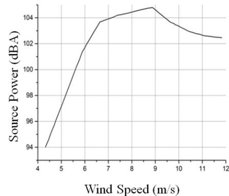
**Fig. 6:** Source power level as a function of the wind speed of a turbine Vestas V52, with height of the hub 65m [34].
