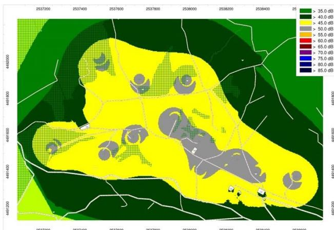
**Fig. 33:** Noise map of the wind farm area, with maximum wind speed predicted by the SARIMA model. Source Power Level: 100.7 dBA.
