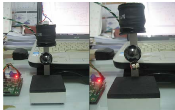
(a) without disturbance (b) with disturbance Fig. 7 Proposed magnetic levitation system
