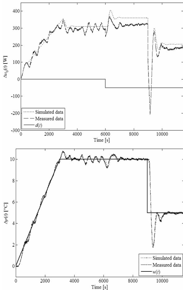
Fig. 9 Measured vs. simulated control responses of  $\Delta u_0(t)$  (left) and  $\Delta y(t)$  (right) for the TFC structure with controllers (27)
