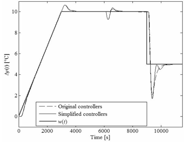
Fig. 7 Simulation control responses of  $\Delta u_0(t)$  (left) and  $\Delta y(t)$  (right) for the TFC structure with controllers (17) vs. (27)
