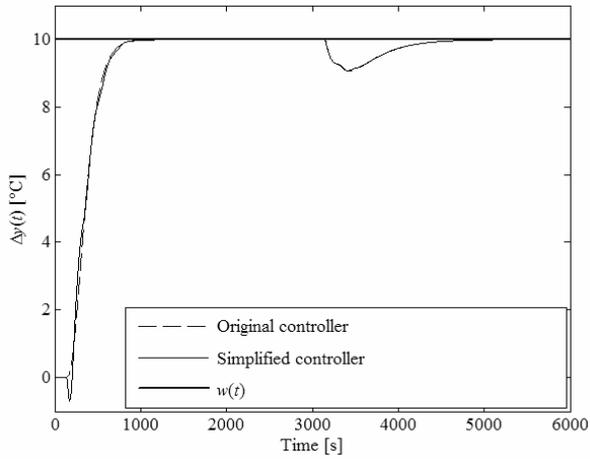
Fig. 6 Simulation control responses of  $\Delta u_0(t)$  (left) and  $\Delta y(t)$  (right) for the simple feedback structure with controllers (16) vs. (26)
