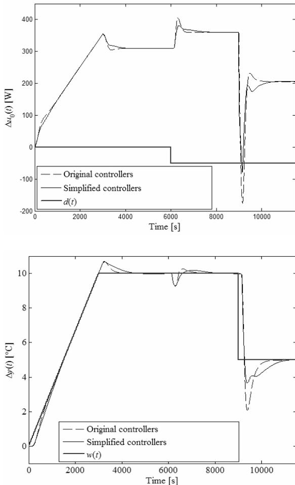
Fig. 5 Simulation control responses of  $\Delta u_0(t)$  (left) and  $\Delta y(t)$  (right) for the TFC structure with controllers (17) vs. (23) and (25) (with a reduced gain)
