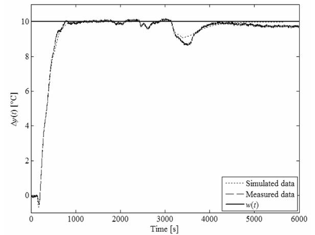
Fig. 8 Measured vs. simulated control responses of  $\Delta u_0(t)$  (left) and  $\Delta y(t)$  (right) for the simple feedback structure with controller (26)
