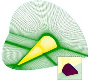
Fig. 2 Typical  $M=5.0$  grid for pitched short protuberance fixed to the blunted cone.
