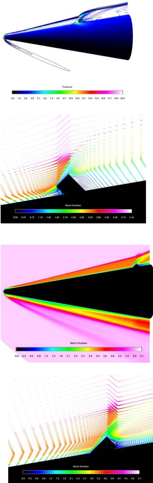
Fig. 5 Pressure contours and velocity vectors for lateral protuberance at 45 degrees pitched forward at Mach 5 and Mach and velocity contours for Mach 6 for 45 degrees pitched aft protuberance.
