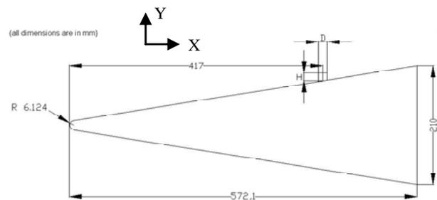
Fig. 1 Blunted cone configuration with lateral short plate.
