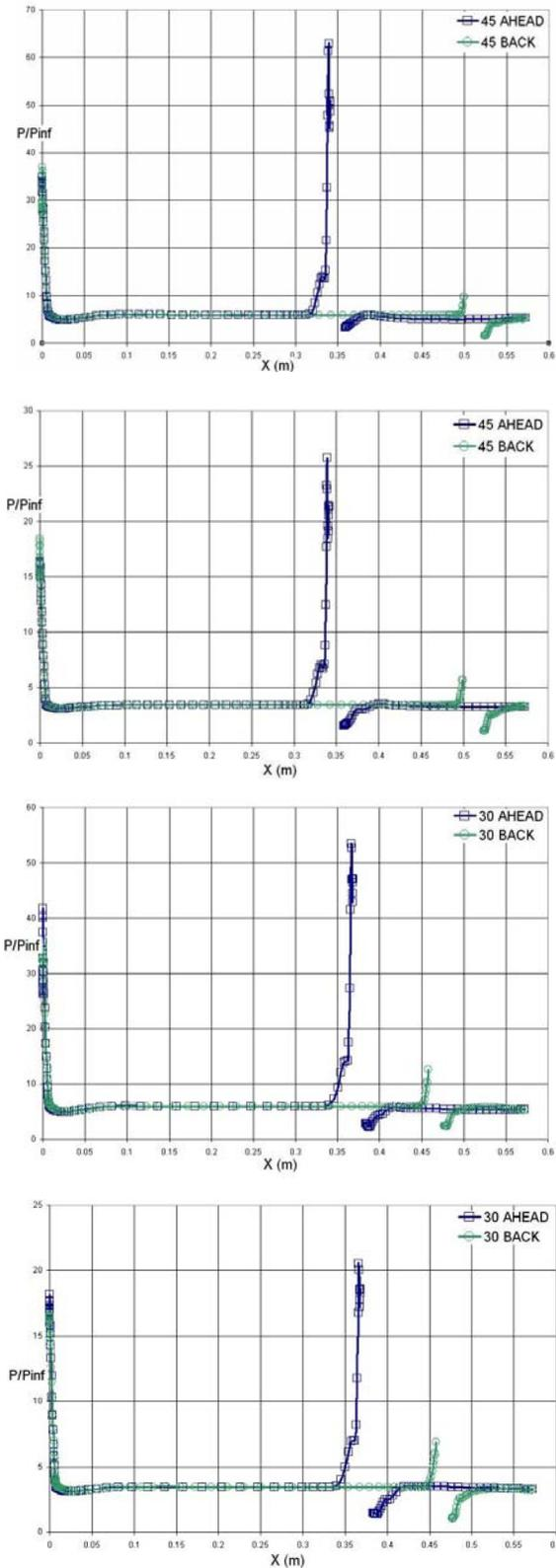
Fig. 3 Leeward surface axial pressure distribution for pitched 45 and 30 deg plate at Mach 5.0 and 3.5 respectively at  $\alpha = -12$ degrees.
