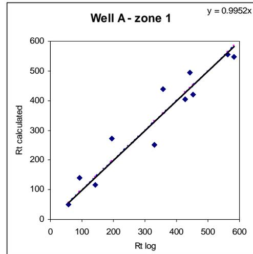
Fig. 1: Comparison of calculated resistivity values with log measurements for the first zone of well A; Correlation 0.96.
