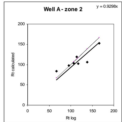
Fig. 2: For the second zone of well A; Correlation 0.88 (dashed line represents the x=y line; solid line is the linear trend line).
