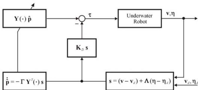
Fig. 1 Diagram showing the parameter adaptation law
