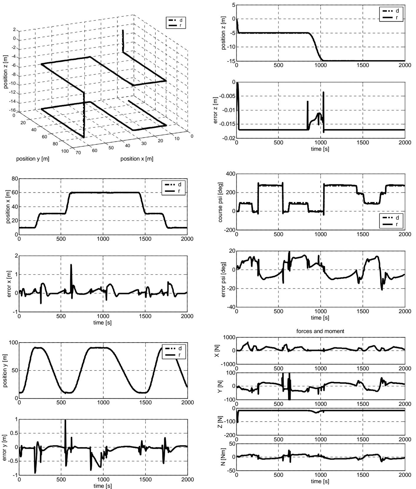
Fig. 3 Track-keeping control under interaction of sea current disturbances (maximum velocity 0.3 m/s and direction  $135^{\circ}$ ): desired (d) and real (r) trajectories (left upper plot), x-, y-, z-position and their errors ( $2^{nd} \div 4^{th}$  plots), course and its error ( $5^{th}$  plot), commands (right low plot)
