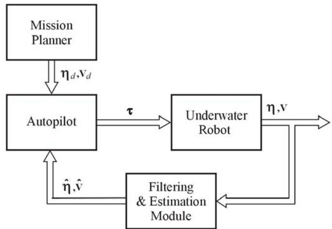
Fig. 2 Main parts of the control system
