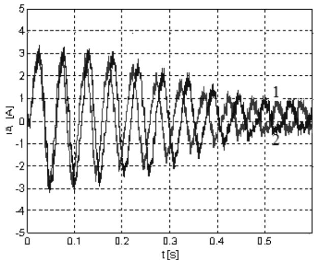
Fig. 7 Graphics dependences corresponding to the cases  $R'_r=5,5 \Omega$  (1) and  $R'_r=4,5 \Omega$  (2)
