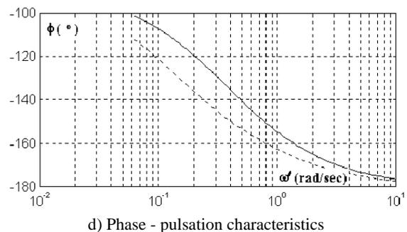
Fig. 2 Graphic dependences corresponding to the cases  $R_s=7,5 \Omega$  (continuous line) and  $R_s=2,5 \Omega$  (dotted line)
