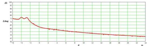
Fig. 24 Radial noise level distribution simulate for a combine.
