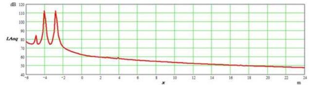
Fig. 25 Radial noise level distribution simulate for a combine.
