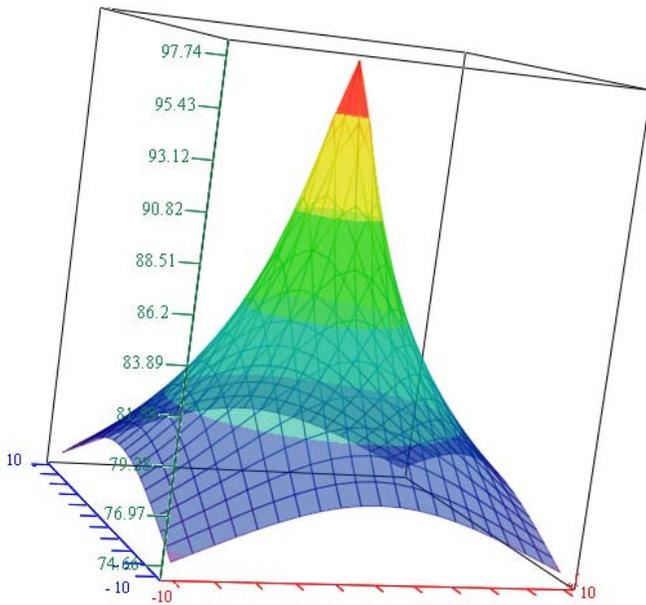
Fig. 22 Noise field mapping for a tractor U-650.
