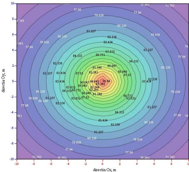
Fig. 23 Noise field mapping for a tractor U-650.
