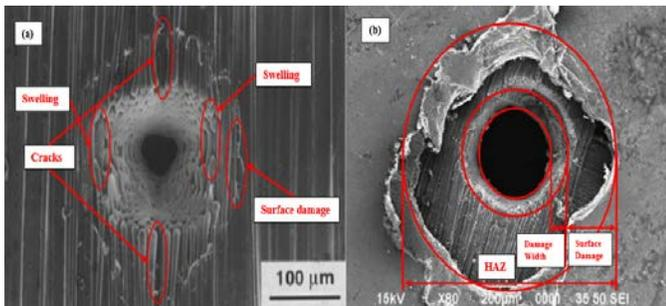
Fig. 5 SEM images of a laser drilled hole indicating the fiber swelling and the damaged areas
