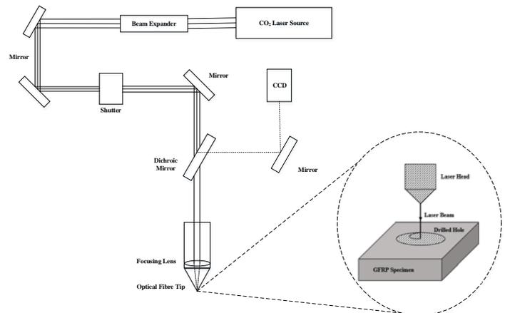
**Fig. 1 Schematic Diagram of CO<sub>2</sub> Laser Drilling**
