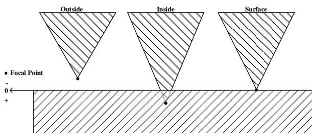
**Fig. 3 Positioning of the focal point**
