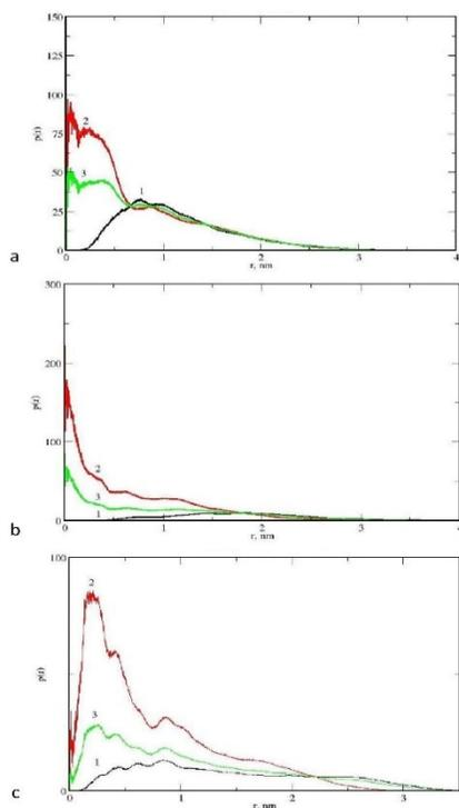
Fig. 6. Radial distribution  $p(r)$  curves: dendrigraft DG2 and 8 Semax (a), dendrigraft DG2 and 16 Semax (b), dendrigraft DG2 and 24 Semax (c). Distribution curves: peptide atoms (1); dendrimer atoms (2); all atoms of complex (3)
