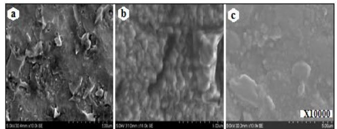
Fig. 7 SEM structure at 220mm/min (a) HAZ-Ti side (b) FZ (c) HAZ-Al side
