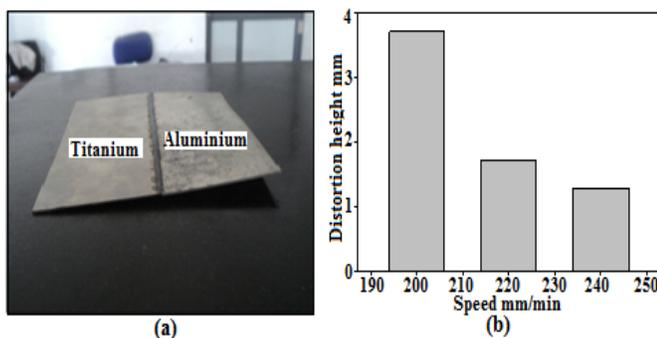
Fig. 5 (a) Maximum distortion at room temperature (b) Effect of distortion on welding speed
