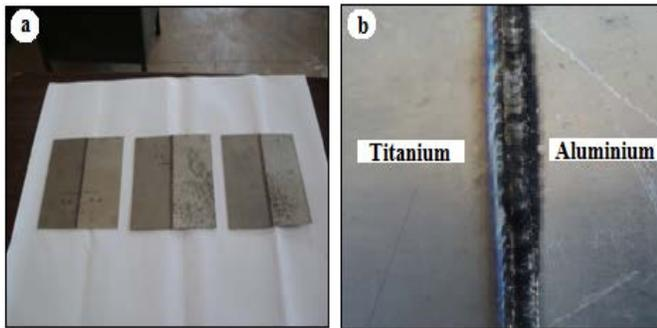
Fig. 4 (a) Macrostructure of the weldment (b) Weld bead
