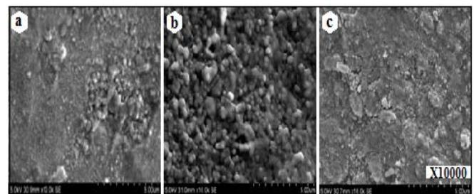
Fig. 8 SEM structure at 240mm/min (a) HAZ-Ti side (b) FZ (c) HAZ-Al side
