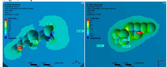
Fig. 9. Thermal growth and inner pressure stress inside closed pore of refractory concrete.
