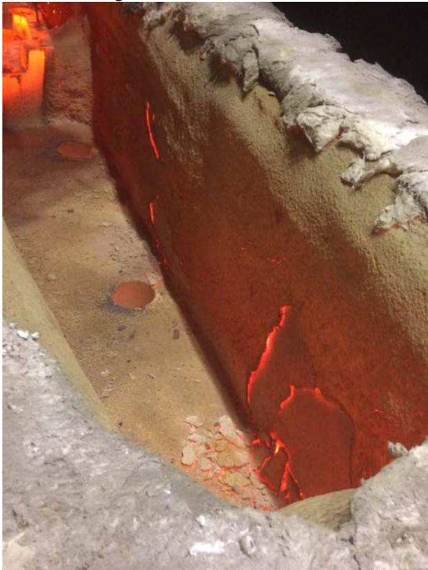
Fig. 8. Gunning mass chipping, while preheating process.
