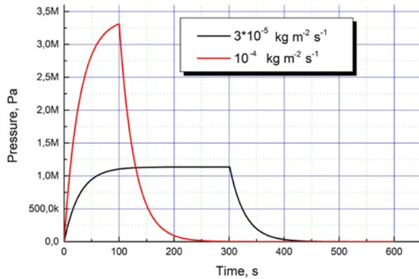
Fig. 7. Water vapor, formed of  $\text{Mg}(\text{OH})_2$  decomposition, pressure, depending on decomposition rate.
