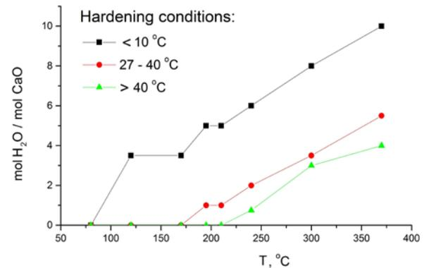
Fig. 1. Free humid formation while thermal dissociation of calcium hydro aluminates, depending on concrete hardening temperature.
