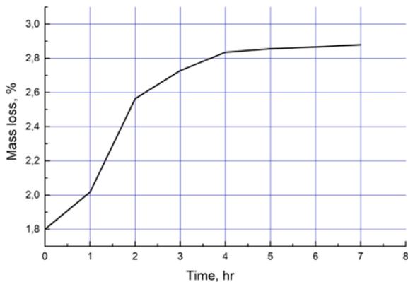
Fig. 5. Typical mass loss graph for refractory concrete (experimental).
