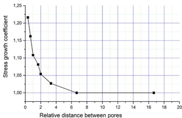
Fig. 10. Coefficient of stress growth dependence on relative distance between pores.
