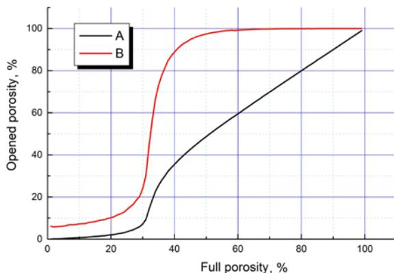
Fig. 3. Full and open porosity obtained with percolation model: A - absolute open porosity value, B - open - full porosity ratio.
