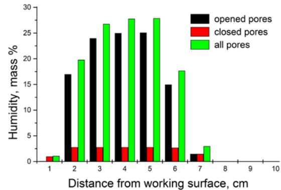
Fig. 6. Calculated humidity of lining working layer after 5 hours exposition (gunning mass was applied to the wall with surface temperature 200 °C).
