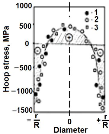
Fig. 2 Residual hoop stress distribution in cylindrical specimens when quenching intensively in water flow or by moving sprayers
