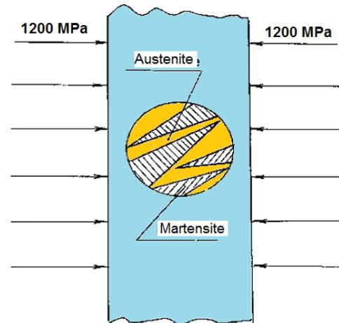
Fig. 3 The transformation scheme of austenite into martensite in the compressed layer, illustrating the effect of additional strengthening (super-strengthening) of the material
