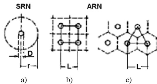
Fig. 5 Possible ways of hollows arrangement in sprayers [21].
