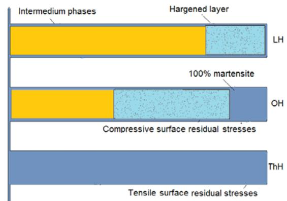
Fig. 1 Optimal depth of hardened layer corresponding to the maximum surface compressive residual stresses: LH, low hardenability steel; OH, optimal hardenability; ThH, through hardening
