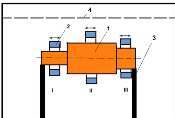
Fig. 4 Apparatus for hardening of large steel parts consisting of two sectioned sprayers moving periodically along the axis in areas I, II, and III: 1 is rotor; 2 is sprayer, 3 is fixture; 4 is water level [20].
