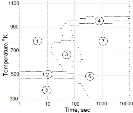
Fig. 10 CCT diagram used for FEM calculations: 1 is austenite; 2 is martensite; 3 is bainite; 4 is pearlite; 5 is martensite after full transformation; 6 is bainite after full process transformation; 7 is pearlite after full process transformation
