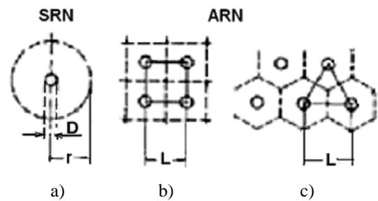
Fig. 5 Possible ways of hollows arrangement in sprayers [21].
