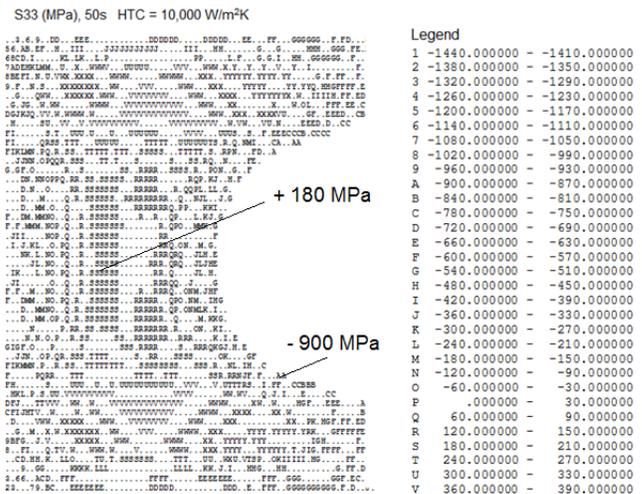
Fig. 12 Hoop stresses distribution in MPa in the roller (see Fig. 9).
