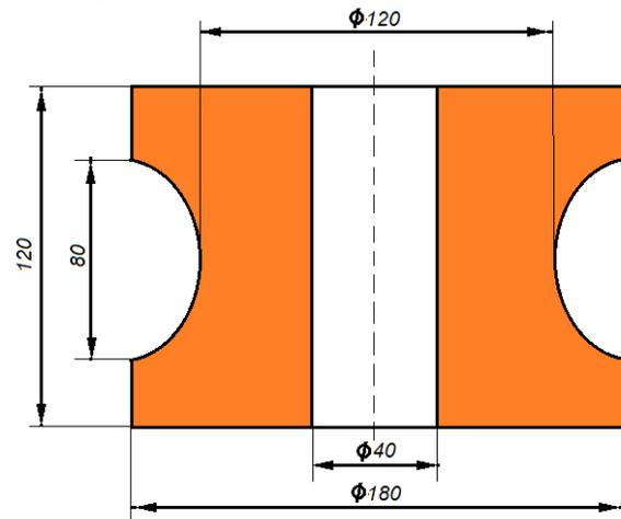
Fig. 9 Drawing of a roller used for FEM calculations
