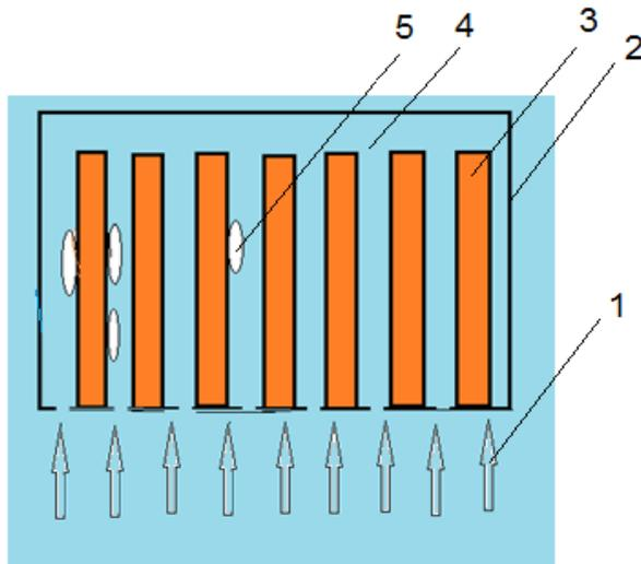
Fig. 8 A load of cylindrical steel parts prepared for batch quenching in the integral quench 36"x36"x72" atmosphere furnace: 1 is water flow; 2 is container; 3 is cylindrical steel part; 4 is quenchant; 5 is local film boiling.[24, 25].
