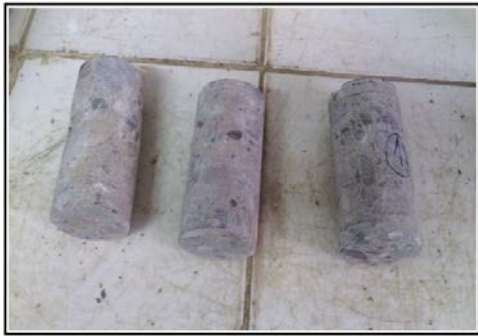
Fig. 4 concrete cylinders (carrots).
