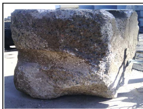
Fig. 2 GCB of 4 \text{ m}^3 retrieved from seawater.
