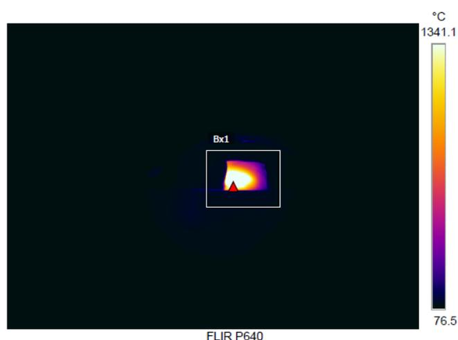
Fig. 9. Infrared image of examined detail with ZnSe glass at 1749,5 °C.
