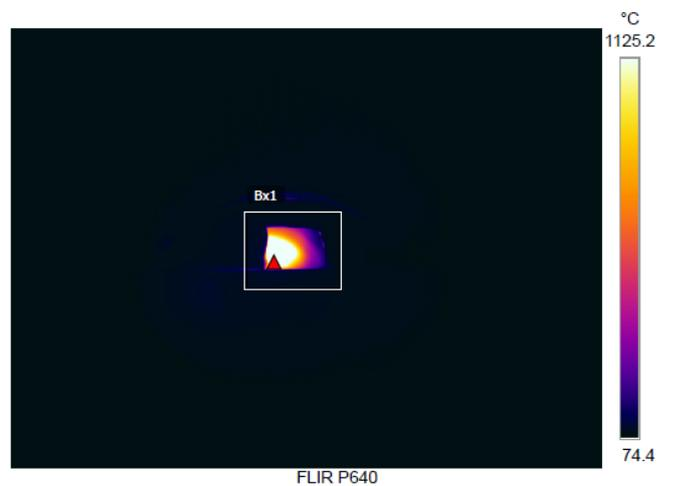
Fig. 8. Infrared image of examined detail with ZnSe glass at 1650,4 °C.
