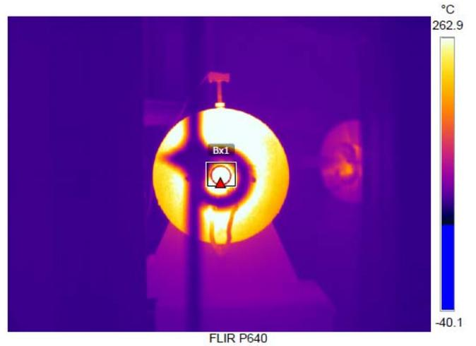
Fig. 7. Infrared image of examined detail with ZnSe glass at 1084 °C.
