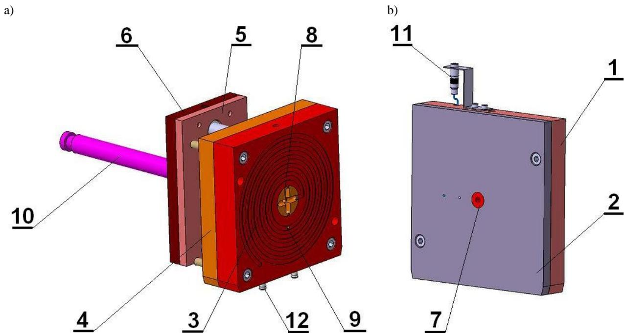
Fig. 3 Shaping part of the injection mold
