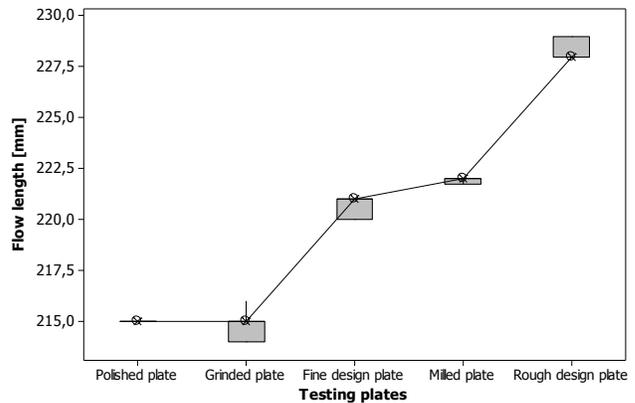
Fig. 12 Influence of the flow length on surface quality (5% glass fibers)
