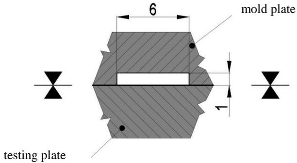
Fig. 4 Cross section of mold cavity
