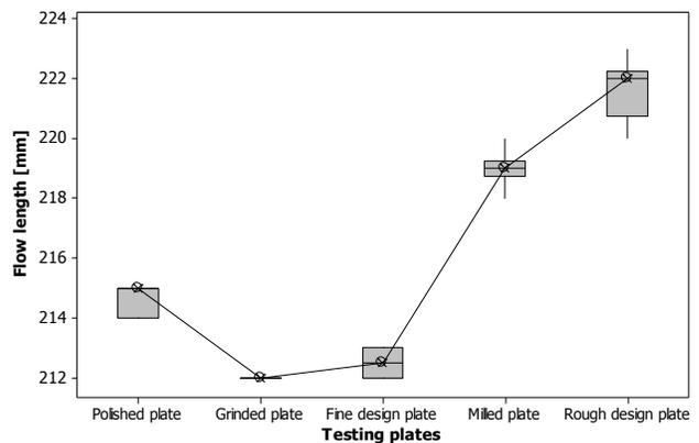
Fig. 13 Influence of the flow length on surface quality (10% glass fibers)
