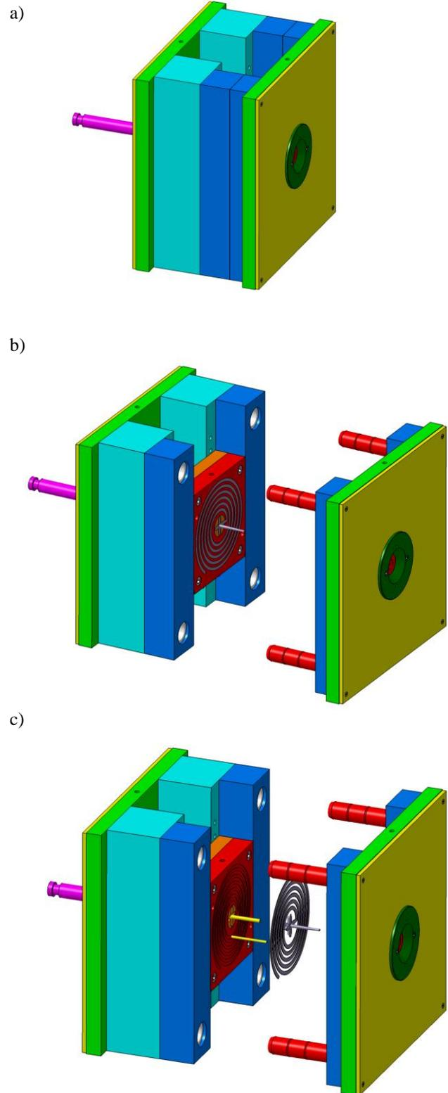
Fig. 9 Injection molding cycle
