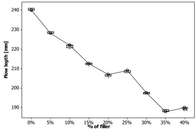
Fig. 24 Influence of the flow length on filler amount (Rough design plate)
