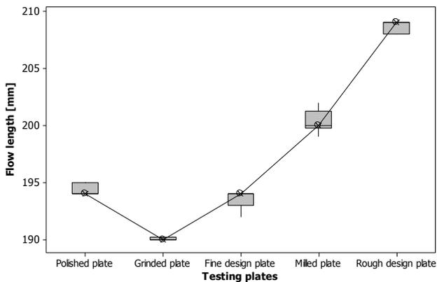
Fig. 16 Influence of the flow length on surface quality (25% glass fibers)
