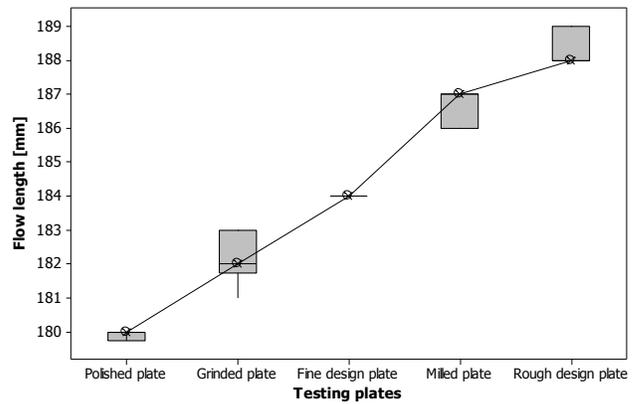
Fig. 18 Influence of the flow length on surface quality (35% glass fibers)
