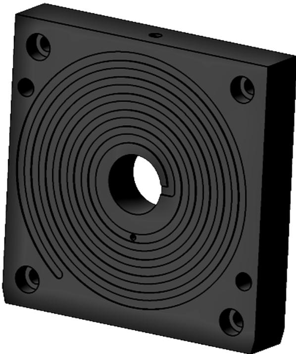
Fig. 5 Cavity plate – shaping plate
