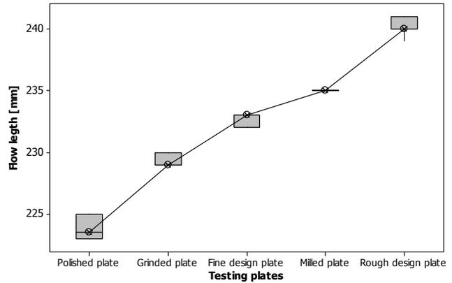
Fig. 11 Influence of the flow length on surface quality (0% glass fibers)
