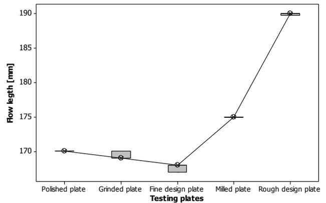
Fig. 19 Influence of the flow length on surface quality (40% glass fibers)
