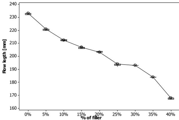
Fig. 22 Influence of the flow length on filler amount (Fine design plate)
