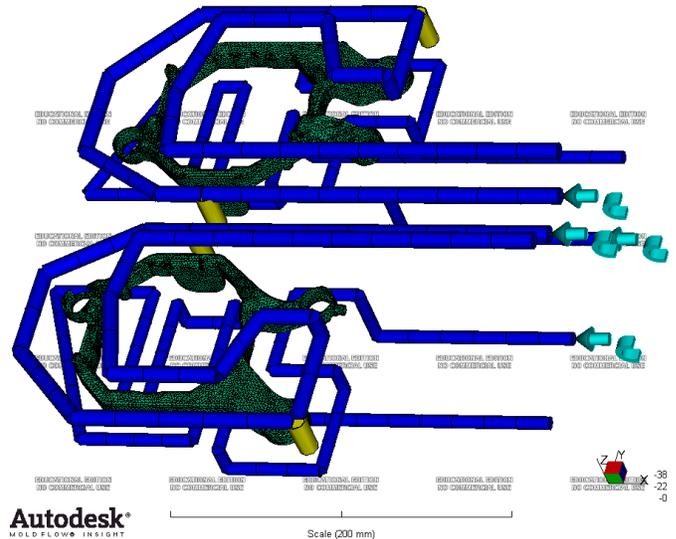
Fig. 10 Cooling system version 3
