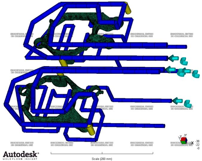
Fig. 10 Cooling system version 3
