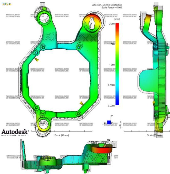
Fig. 12 Product deformation from PBT with gate location version 2 – the highest amount of deformation
