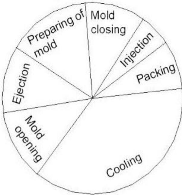
Fig. 1 Injection molding cycle
