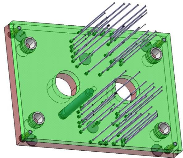
Fig. 11 Ejection system
