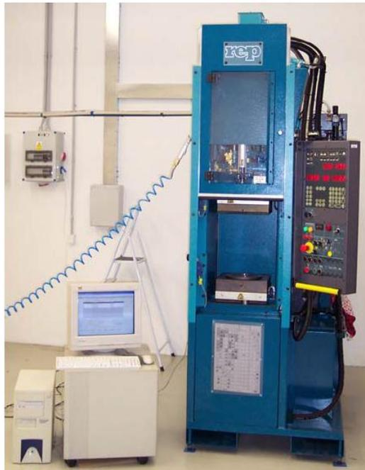
Fig.18 Injection molding machine REP V27/Y125
