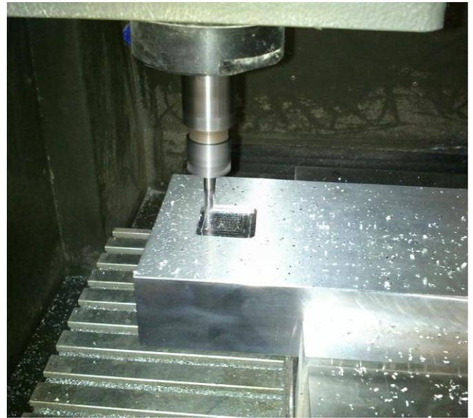
Fig.25 Illustration of manufacturing of cavity
