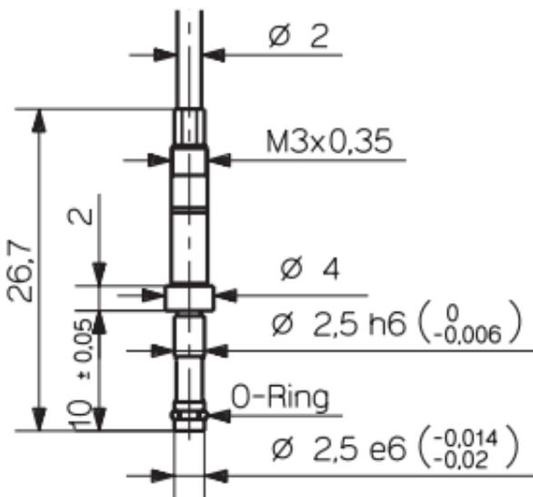
Fig.14 Dimension of sensor
