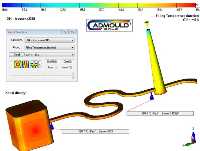
Fig.20 Sample of computational analysis in Cadmould rubber software
