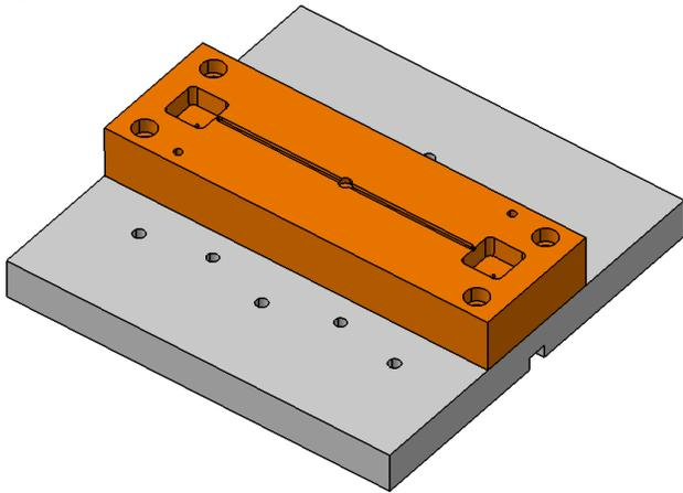
Fig.6 Universal frame with cavity plate (lower part)
