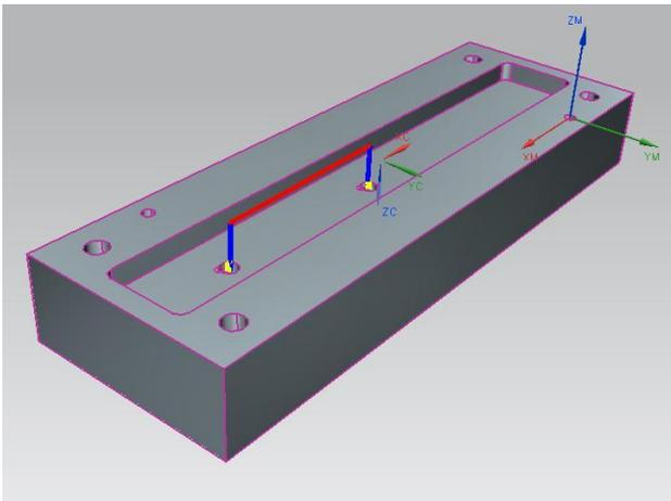
Fig.13 Drilling holes for sensors
