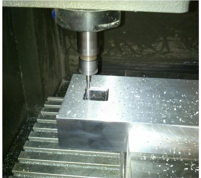
Fig.25 Illustration of manufacturing of cavity
