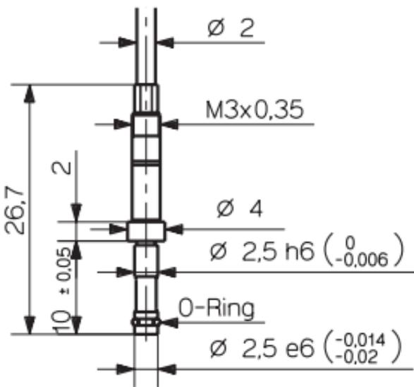
Fig.14 Dimension of sensor
