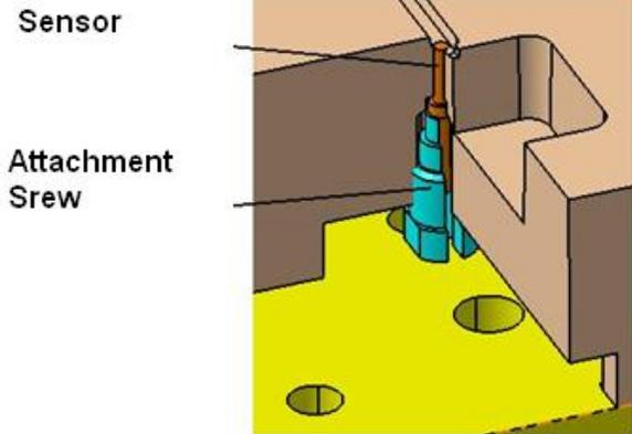
Fig.15 Attached sensor in runner
