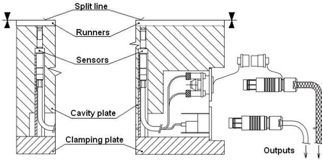
Fig.17 Situation sensors in mold
