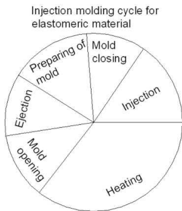
Fig.2 Elastomeric injection molding cycle
