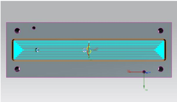
Fig.12 Roughening space for sensors
