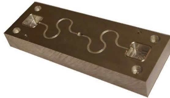
Fig.8 Manufactured cavity plate
