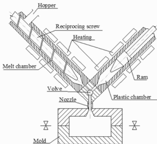
Fig.19 Schema of REP V27/Y125 machine
