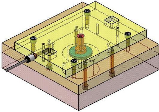
Fig.5 Model of upper part of mold
