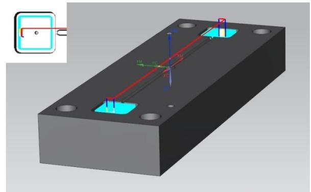
Fig.10 Finishing of cavity
