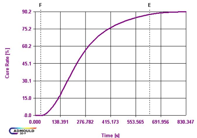
Fig.21 Sample of Cure curve Cadmould rubber software for this issue
