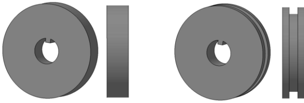
Fig. 3. Testing sample for fast wear test a) Before the test, b) after the test
