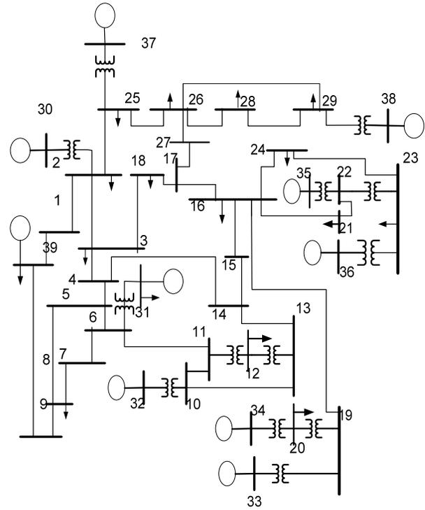
Figure 10: One-line diagram for the New England system
