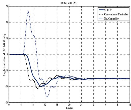
Figure 11 Angle deviation of (G30-G39)
