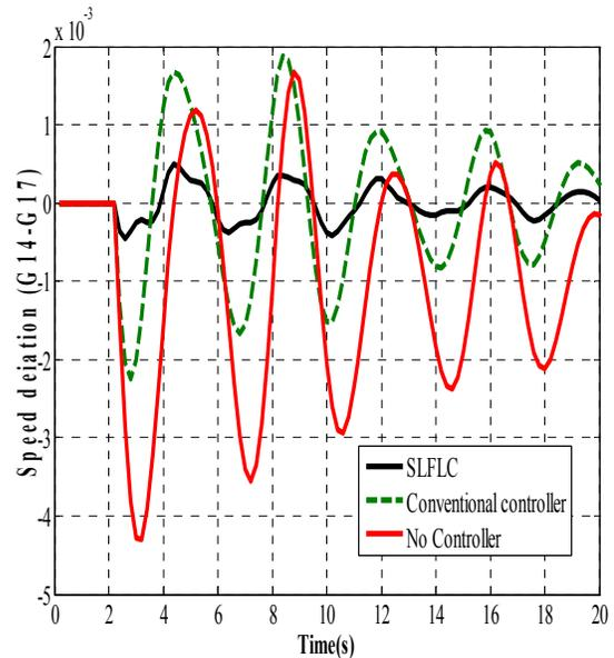
Figure 7 Speed deviation of (G14-G17) for line 7-10 outage
