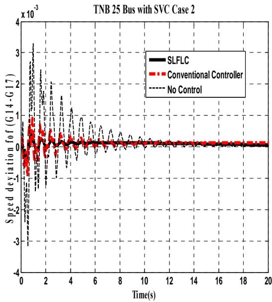
Figure 8 Speed deviation of (G14-G17) for line 8-12 outage
