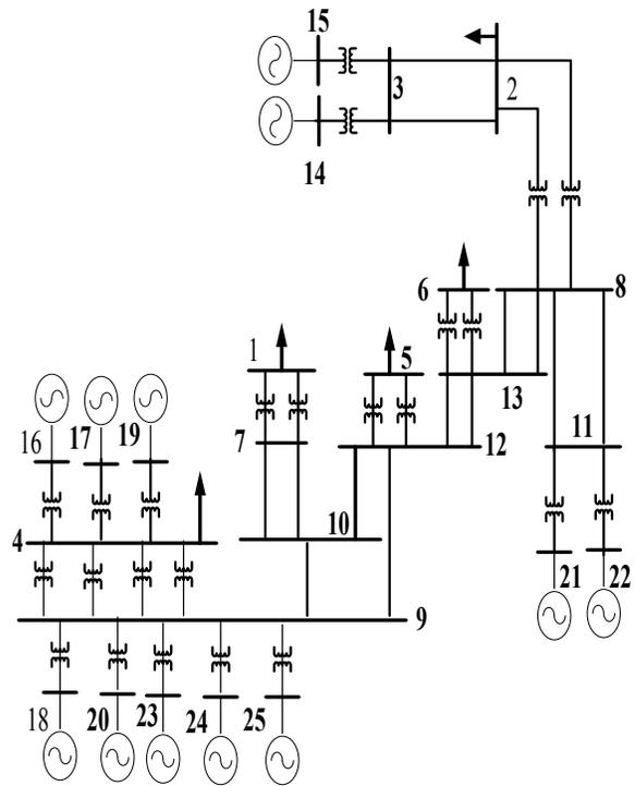
Figure 6: 25 Bus equivalents of South Malaysian Network
