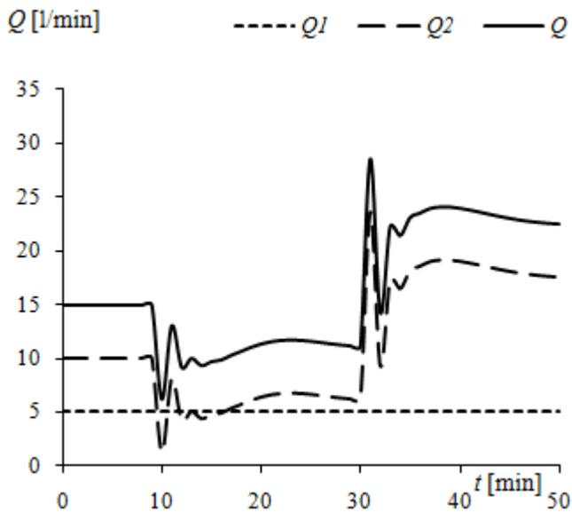
Fig. 16 Simulation model of PID controller – time dependencies of action signal  $Q_2(t)$ ,  $Q_1(t)$  and  $Q(t)$
