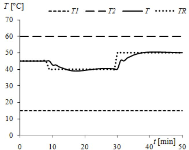
Fig. 15 Simulation model of PID controller – time dependencies of  $T_1(t), T_2(t), T_R(t)$  and  $T(t)$
