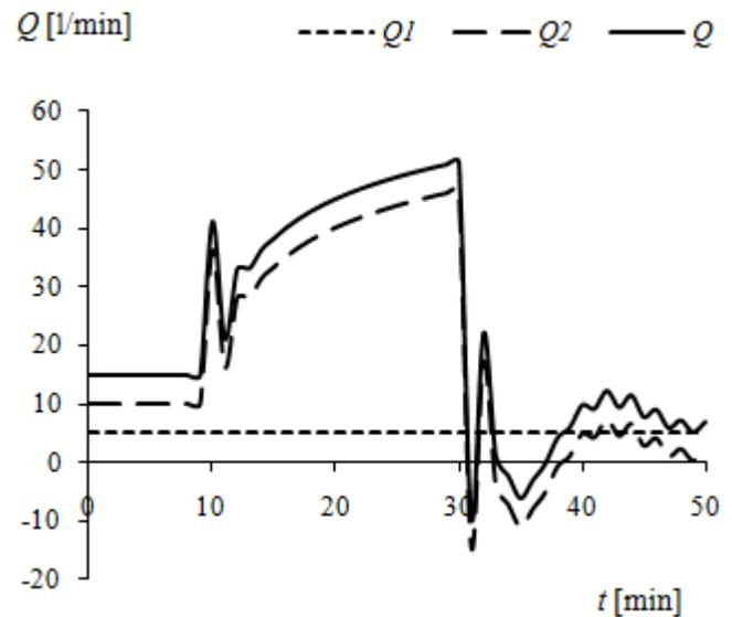
Fig. 18 Simulation model of PID controller – time dependencies of action signal  $Q_2(t)$ ,  $Q_1(t)$  and  $Q(t)$  of non-controllable system
