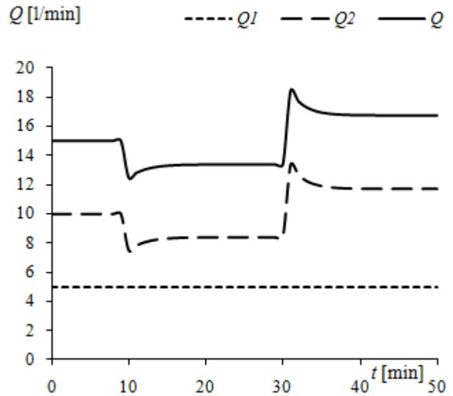
Fig. 14 Simulation model of P controller – time dependencies of action signal  $Q_2(t), Q_1(t)$  and  $Q(t)$
