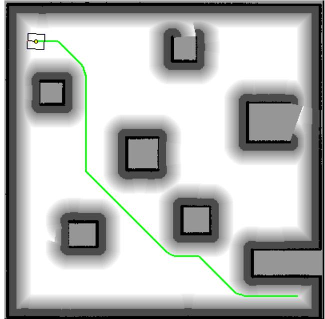
Fig. 8 Optimal path computed by the original algorithm
