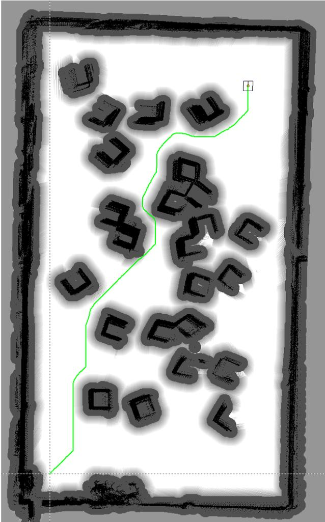
Fig. 12 Motion of the experimental vehicle in the real environment
