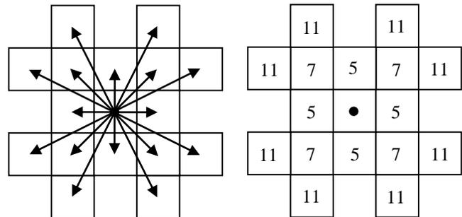
Fig. 5 Graph edges from each node in the grid and their costs
