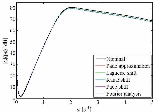
Fig. 4 Bode magnitude plots of the nominal and approximating systems for (28)
