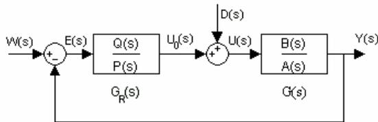
Fig. 2 Simple feedback control loop
