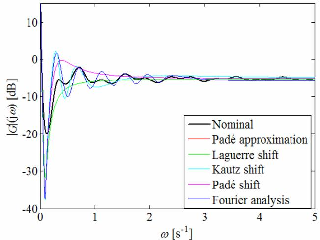
Fig. 2 Bode magnitude plots of the nominal and approximating systems for (22)
