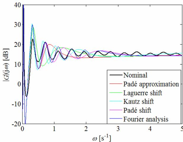
Fig. 3 Bode magnitude plots of the nominal and approximating systems for (24)
