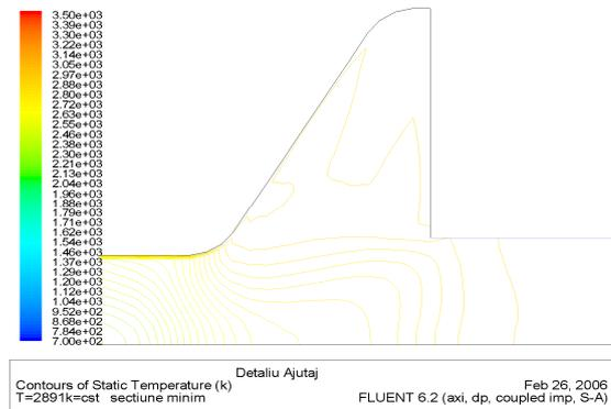
Fig. 3 – 2D study revealing peak  $T= 2,930 \text{ } ^\circ K = cst$  And consequently the simulation for T = variable case will bring next results:
