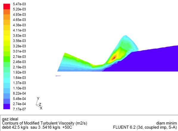
Fig. 14 – 3D study in the convergent nozzle area turbulence issues like results of the initial temperature distribution inside the rocket engine
