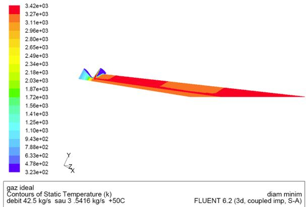
Fig. 11 – 3D study initial flow temperatures because of the initial assumed temperature distribution inside the rocket engine as Table 1
