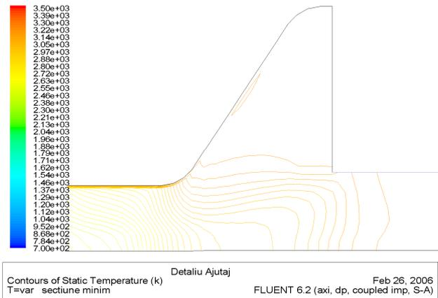
Fig.4 – 2D study revealing peak  $T= 3,430 \text{ } ^\circ K$
