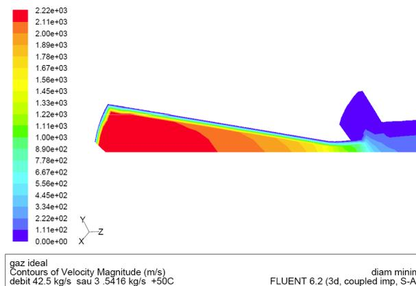
Fig. 13 – 3D study in the nozzle area velocity distribution like results of the initial temperature distribution inside the rocket engine
