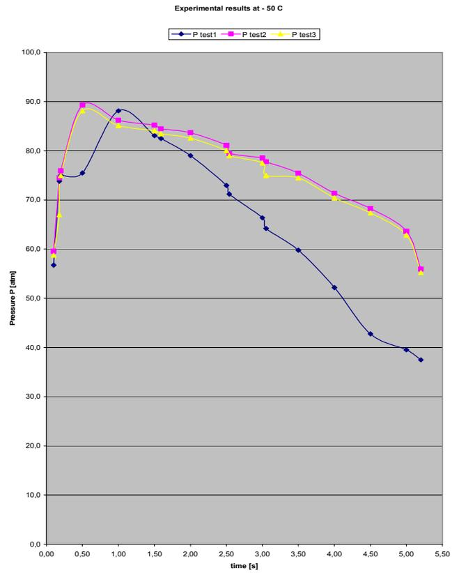
Chart5 - measured values for inside pressure at -50 deg.C
