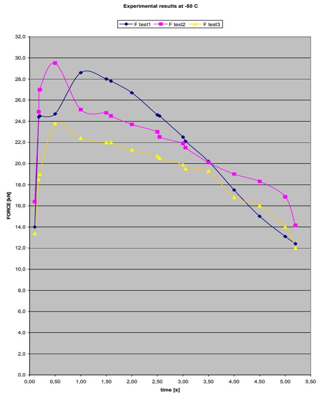
Chart 6 – measured values for thrust force at -50 deg C
