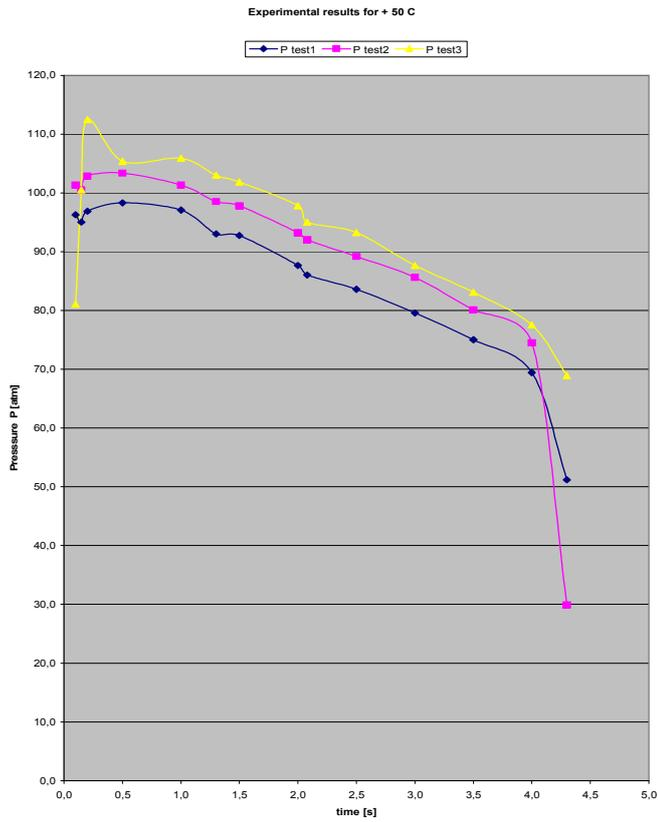
Chart3 - measured values for inside pressure at +50 deg.C
