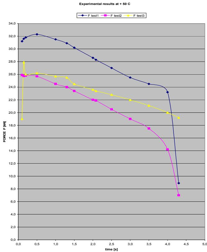
Chart 4 – measured values for thrust force at +50 deg C
