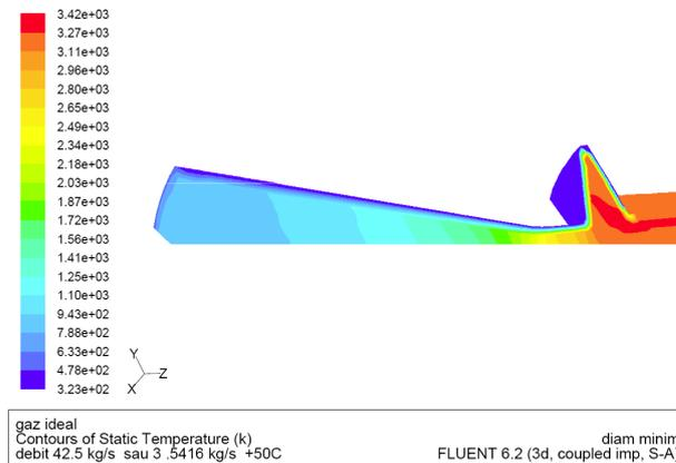
Fig. 12 – 3D study in the nozzle area flow temperatures like results of the initial temperature distribution inside the rocket engine
