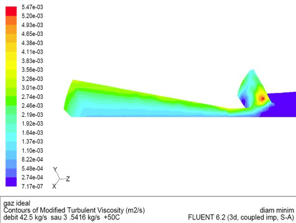
Fig. 15 – 3D study in the divergent nozzle area turbulence issues like results of the initial temperature distribution inside the rocket engine
