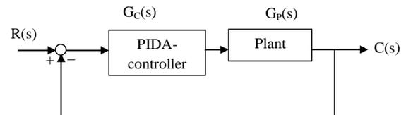
Fig. 1 A closed-loop system.
