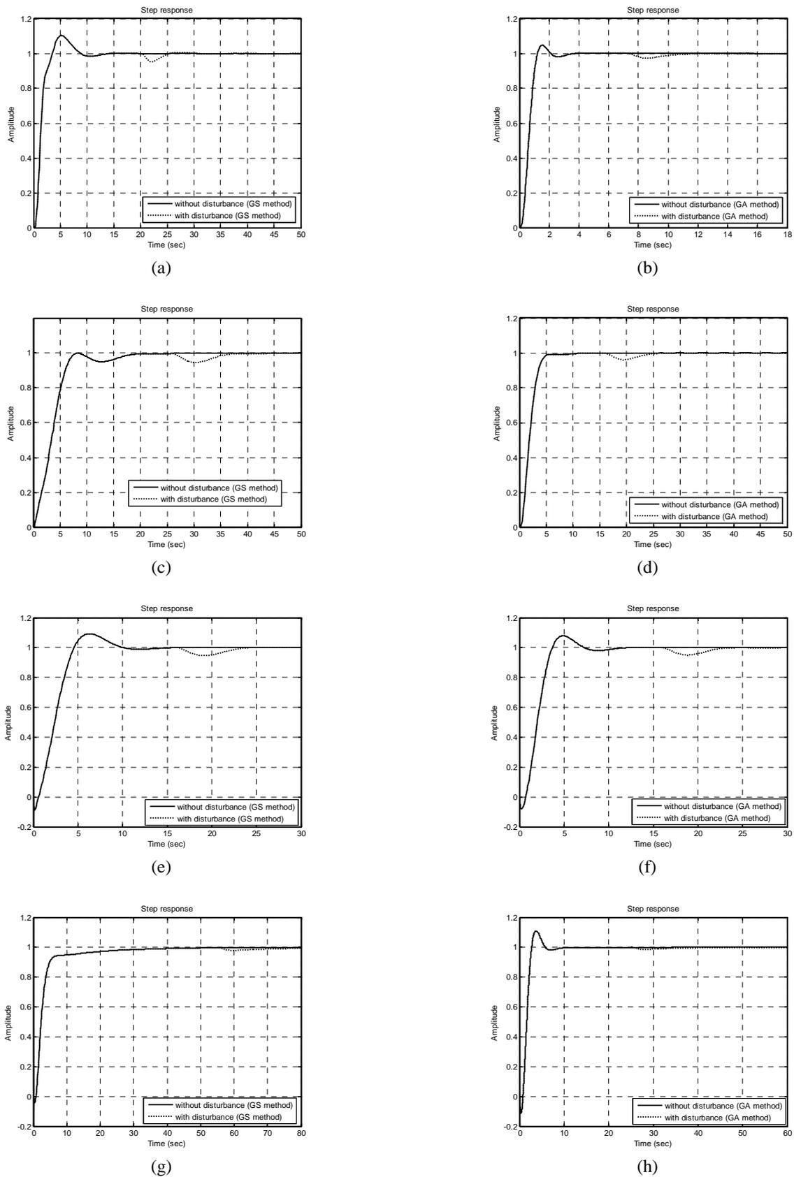
Fig. 6 Responses to step inputs and disturbances (GS and GA methods).
