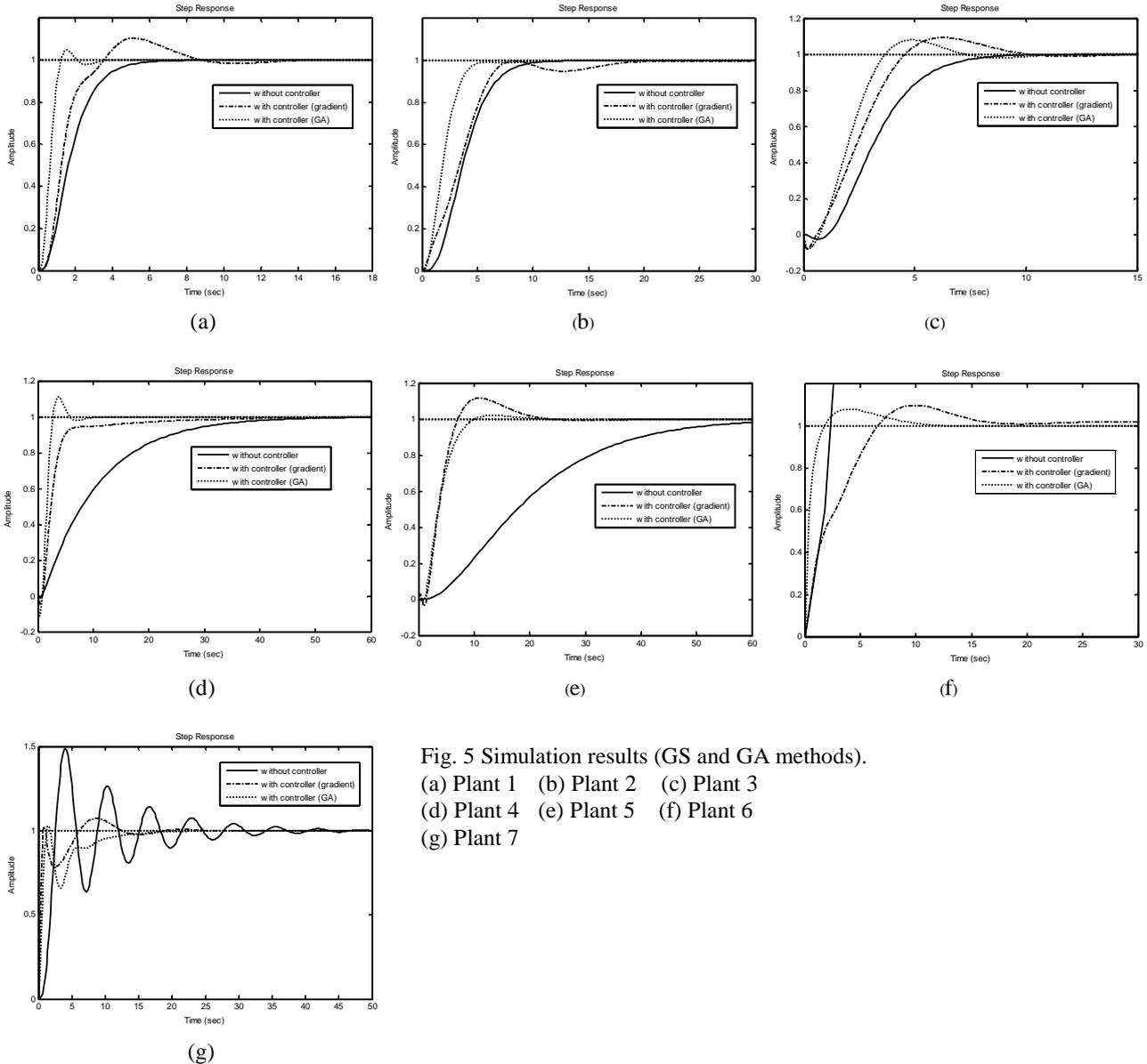
Fig. 5 Simulation results (GS and GA methods).
