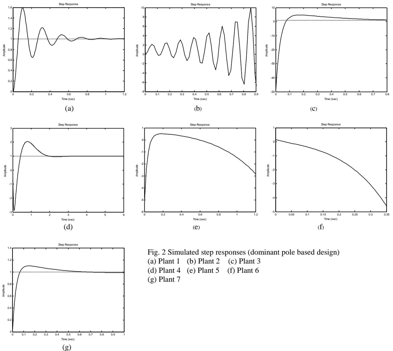
Fig. 2 Simulated step responses (dominant pole based design)
