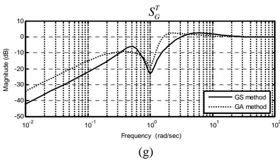
Fig. 7 Sensitivity functions ( $s_G^T$ ).
