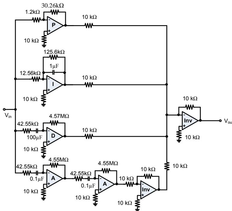
Fig. 9 Analog implementation of the controller.
