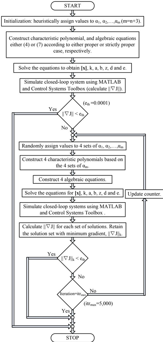
Fig. 3 Flow diagram of the GS method.
