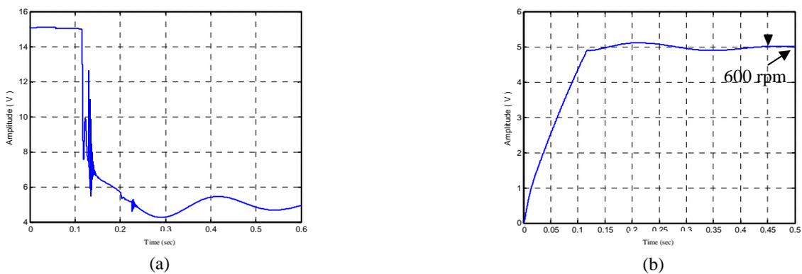
Fig. 11 PSIM results (a) control signal, (b) motor speed.
