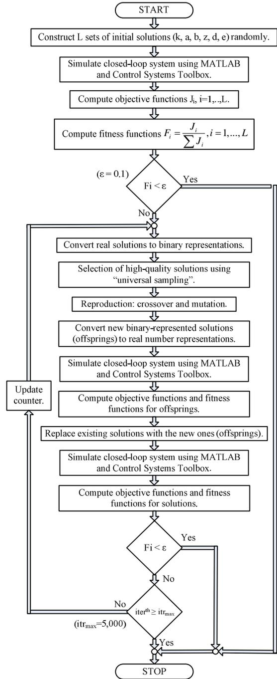
Fig. 4 Flow diagram of the GA method.
