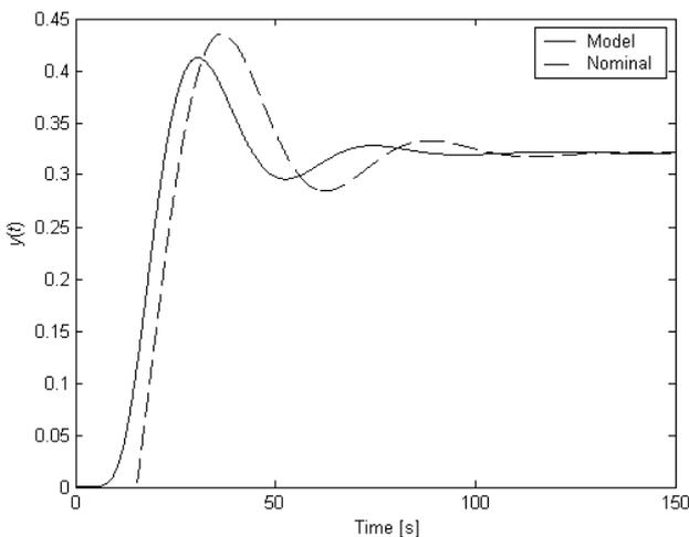
Fig. 7 Feedback response when control the nominal plant (44) and the model (45) by a proportional controller  $q = 0.473$
