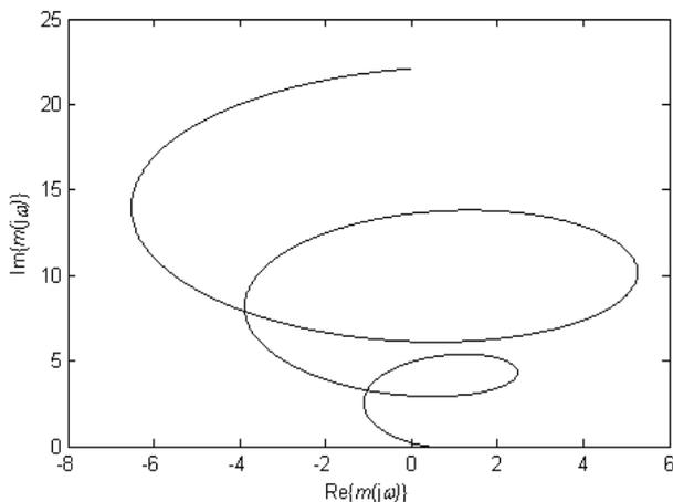
Fig. 4 Mikhaylov plot of the stabilized quasipolynomial,  $\omega \in [0, 15]$  - Example B
