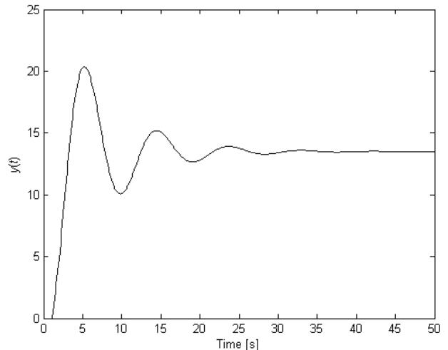
Fig. 5 Proportionally stabilized feedback response – Example B
