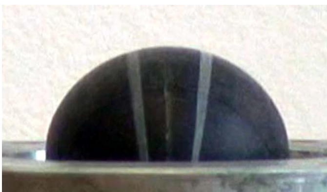
Fig. 6 inflated equibiaxial specimen with white stripes
