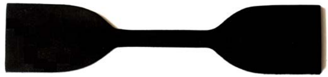
Fig. 4 1A type of uniaxial tension test specimen (ISO 37)
